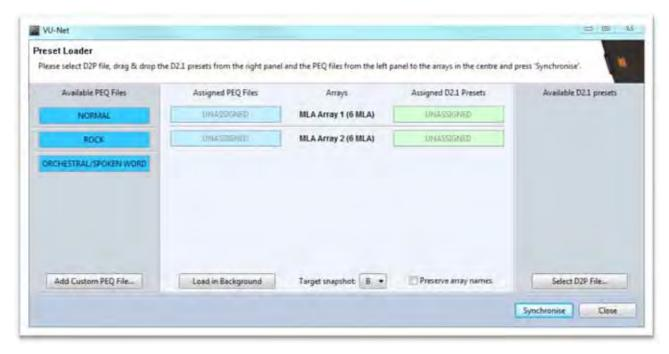
The first stage is to load the D2P file created for the project using Display 2.1. Click on the 'Select D2P File' button and navigate to the file location.
