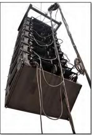
When you arrive at the final cabinet the only difference is that the trailing second U-Net cable is connected to the final U-Net 2 port on the last cabinet and the U-Net LED should be checked for good network connectivity between the final cabinet and U-Net port 2 on the Merlin back in the rack.
