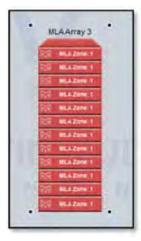
The array is coloured red to show that it is off line. Note that the largest array that can be added is a total of 24 cabinets which matches the maximum flown array from the flying grid. If you enter a number higher than 24 Vu-Net will enter a 24 box array.
