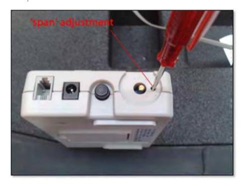
Carefully adjust the pot until the display matches the reference. Next lower the grid to around -30° and -20° checking each time that the reference and reader displays match. It may be necessary to re-adjust the zero measurement following calibrating the span, in which case check the span calibration again.
