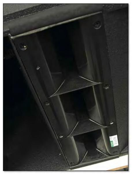
Early proponents of touring line arrays strongly advocated a flat wavefront from each individual HF element. However, our sophisticated in-house BEM (Boundary Element Method) modelling techniques have shown that slightly curved wavefronts deliver much more consistent SPL's to the audience in real-world use where the array is curved.
