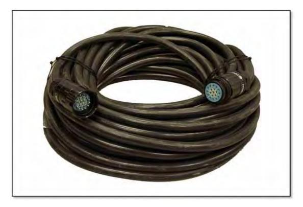
**ASF12002** is a 30m 18-core multiway mains cable terminated with Tourmate 19-pin connectors, one male, one female. Tourmate is based on the popular Socapex pattern but is rated at IP67 when mated so if suitable for use outdoors in all weather. The cable has 18 cores each 2.5mm<sup>2</sup> and has a tough, flexible outer sheath. Other lengths are available to special order. The Tourmate is used to connect a Master or Slave rack to an array.
