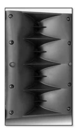
MLA Compact's HF section utilises  $4 \times 0.7$ " (19mm) exit neodymium compression drivers which feed separate horns for true 100° horizontal constant directivity. In the vertical plane, MLA Compact makes significant advances over previous thinking by adopting new criteria for vertical wavefront curvature.
