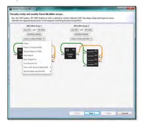
For a larger system the options will change, for example, as the maximum for pole mount is 4 cabinets, 8 or more in an array will remove this option;-
