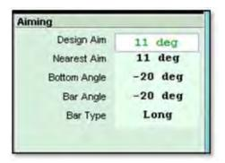
As with Compact there are two types of ground stack bar, a long and a short. For ground stack arrays which require a down-tilt on the bottom enclosure the long bar is used as in the above example, for array which require an up-tilt the short bar is used;
