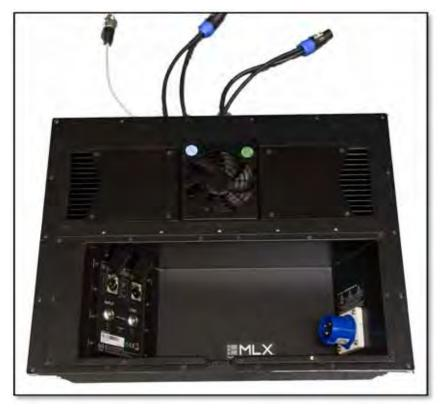
The module is held in place behind the ventilation panel and connector lid, removal is a simple case of unscrewing the fixing screws and disconnecting the two Neutrik NL4's which connect the drivers and LED's to the module, the Neutrik p-pin XLR which connects the iPal pressure sensor and the Cat 5 cable that links to the iPal data port. Field replacement therefore is very quick and easy in the unlikely event of a module failure.
