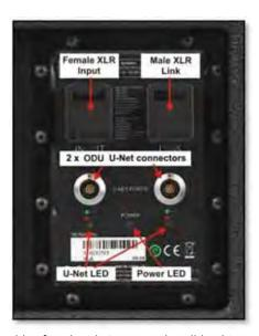
U-Net connections are made using Cat5 cables fitted with 8-way push pull latching connectors compatible with ODU Series K. Robust Cat 5 cable should be used such as Neutrik Etherflex or Belden 1305A, this will ensure reliable network connections of up
