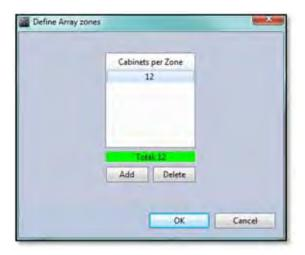
This shows a single zone of twelve cabinets, the total at the bottom is shown in green because it equals the numbers in all zones. We now click 'Add' and an additional zone is added of one cabinet below the first. The upper zone has its quantity reduced to eleven to maintain the total of twelve;-
