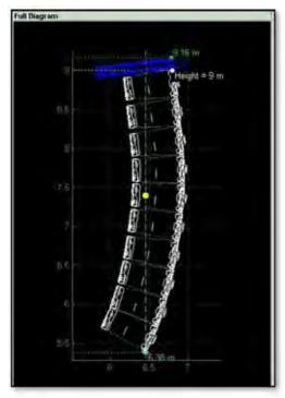
This is useful so you can quickly see if there are any mechanical issues with the array that might make flying in a particular venue difficult; perhaps the rear of the array is hanging back further than you initially thought and might impede something else that
