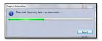
The meter bar will gradually move across until it is completely green and all devices have been found. This may take a few seconds on large systems with large arrays of many cabinets.
