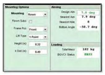
The first option for mounting determines how the array is to be deployed Using the Mounting drop-down;-
