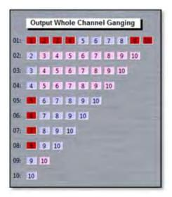
You can see that the red squares by the channels that have been ganged have disappeared from the vertical column and are now in the horizontal line from channel one. You will see on the part ganging screen that all parameters for the ganged channels are now coloured red to indicate that they are all ganged together;-
