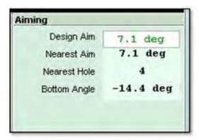
Note that if by a happy coincidence the 'Nearest Hole' gives an angle which happens to match the Design angle the identical angles will automatically be green.
