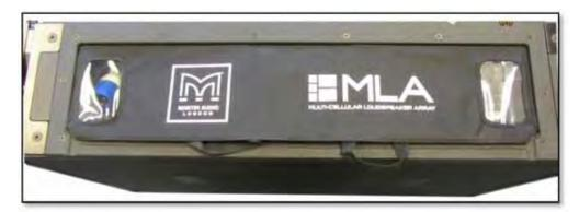
The cowl travels folded flat for ease of transportation. It is held in the operating position by two triangles of canvas mounted towards the middle of the cowl. These have straps attached and by pulling the straps the cowl pops up into position and is held in place with the two supporting triangles which connect to the inside of the cowl using Velcro. To fold the cowl flat, the straps are again used to pull the supporting triangles down left and right.
