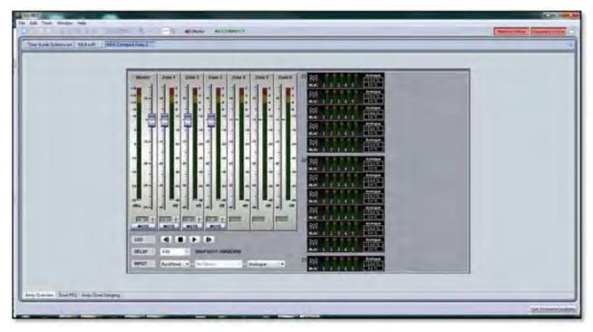
This page is the Array Overview; each array also has a tab for Zone PEQ and Ganging. First we will look at the metering and gain faders. Here is a 12 box array that has been divided into three zones, the top five cabinets, next six and an MLD. The Master and Zone Section looks like this;-
