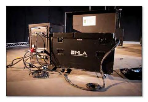
Connect the Tourmate mains cable to the mains distro, U-Net cables to U-Net ports 1 & 2 on the patch panel and the inclinometer cable to the reader which can be placed on top of the rack. If you are using the Merlin in the rack for audio distribution you can connect the array audio feed to the relevant audio output on the patch panel;-
