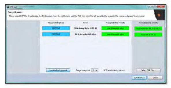
The PEQ already uploaded will be preserved and if you select an alternative snapshot to the one currently being used you can even synchronise while the system is in use. It will synchronise in the background as the name suggests without disturbing system performance and you can then wait for an appropriate break in a show or rehearsal to select the new snapshot.
