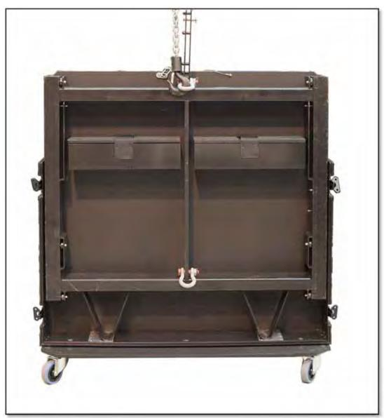
At this stage if you are flying from a single point add a second shackle to the required rigging point as calculated by the rigging spreadsheet and switch the hoist chain from the rear point to the middle. It is advisable to do this with a second person to support the grid as it will be completely unsupported without the chain attached.
