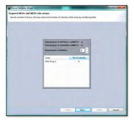
If you have more than one array of each type of cabinet on the same U-Net loop you have the opportunity to divide them into two or more arrays as required. Use the up/down button to select the number of arrays then change the number of cabinets in each array to match what you physically have connected;-
