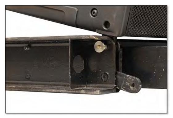
Now connect the MLA ground stack bars to the appropriate holes in the grid just under the rear of the MLA. Raise the rear of the cabinet and pin the bar into the hole in the MLA as required to obtain the necessary angle;-
