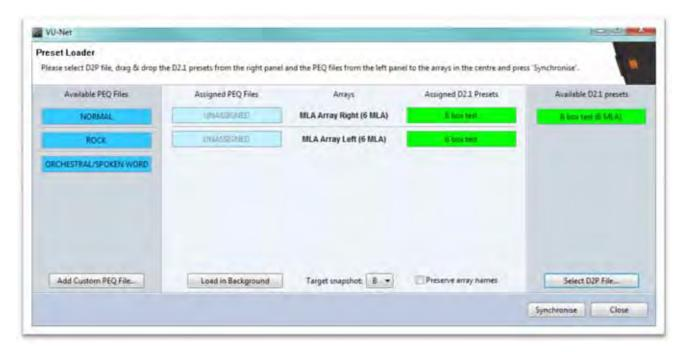
As we may not want to disturb the arrays that are working perfectly well we may want to just upload the optimisation to the new array with the module we have replaced. In this case drag the optimised file out of the array back to the "Available D2.1 presets" position and you will have the following;-
