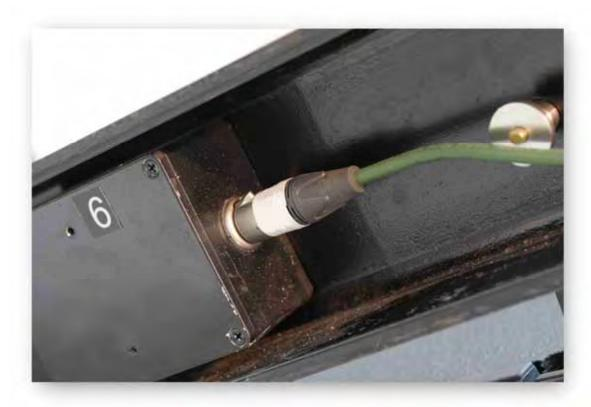
Connect one of the 800mm AES XLR cables and an 800mm U-Net cable (usually loomed together) from the audio out and U-Net port 2 on the top MLA cabinet down to the Audio input and U-Net port 1 on the second cabinet;-
