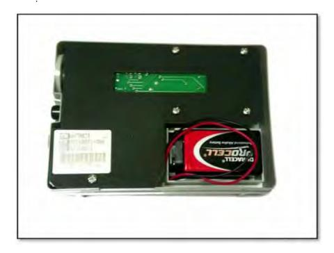
Ease the battery out, pull the clip off the terminals, clip the new battery onto the battery lead and replace it in the upper half of the case. The bottom is fitted back on and clips into place. Turn the reader on to check the new battery has been fitted correctly and is working ok.
