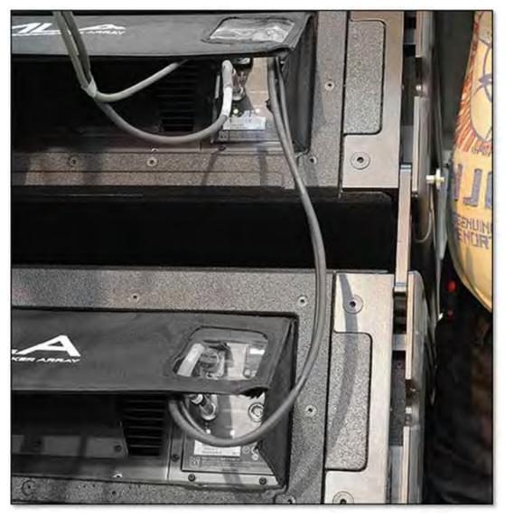
At this point the U-Net ports will not light on either cabinet as the second cabinet is not yet powered.
