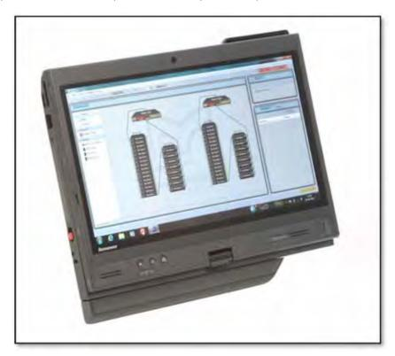
All necessary software is supplied fully installed on the Tablet and it is pre-configured to connect wirelessly with the system Master rack. In addition there are some additional utilities files installed for routine system maintenance. The tablet is supplied in a flightcase which houses its power supply, a Leica Disto D8 laser measure, a U-Net to RJ45 barrel adaptor and with the Mk1 system it also holds the WAP antenna.
