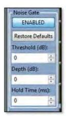
Each amplifier module has an internal noise gate set to keep the amplifier and DSP noise floor as inaudible as possible. By default it is enabled but it is possible that with very low levels of program material the gate operation may be audible and so the gate can be defeated by pressing the ENABLED button. The button will then display 'DISABLED';-
