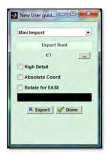
As with Balloon Exports the first stage is to select which of the arrays in your project you wish to Export using the drop-down at the top of the window;-
