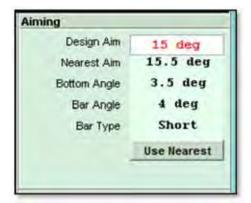
Also in common with MLA Compact, the ground stack bars are labelled with the angles that they can produce so that is shown in the Aiming panel rather than which particular holes in the bar and cabinet to use.
