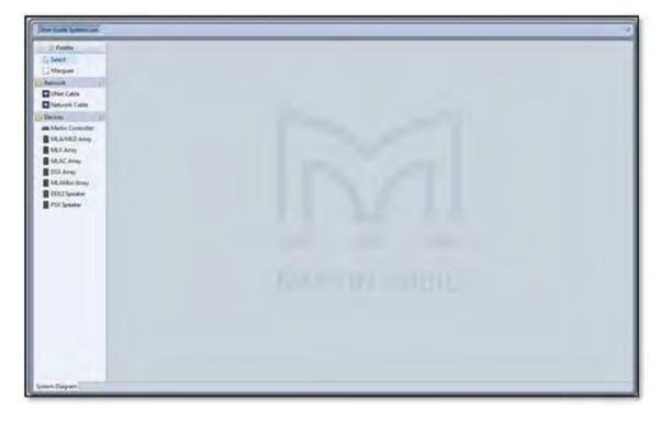
This window will show all array components on the network and is used for all configuration changes and system monitoring. The palette on the left is used to manually enter system components when working off line (in normal use, Device Discovery is used to find all connected components). If you need to maximise the workspace the palette can be minimised by clicking on the white triangle in the top left corner of the palette;-
