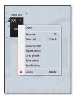
'Open' functions in exactly the same way as double clicking on the cabinet icon and opens the DD12 overview screen to allow detailed control and monitoring
