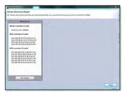
This shows a list of all connected devices found grouped into categories; Merlin Controllers, MLA, MLD, MLX et cetera. Each individual U-Net network created either by a Merlin or USB connected device (such as an MSX or DD12) will create an individual window with the IP address shown at the top. All devices connected to that U-Net loop will be listed grouped by type.
