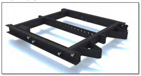
The MLA Compact flying Grid is supplied in pairs with all MLA Compact systems. It enables flying of up to 24 MLA Compact when using a two point lift, or 12 enclosures from a single point. Ground stack systems of up to 6 Compact can also be employed using the same grid with the addition of ground stack bars which as supplied as part of the system.
