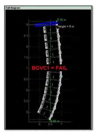
In this case it is necessary to chance the height and possibly coverage area of the array until a "legal" array shape is produced or in the case above, reduce the number of cabinets or switch to a two point hang.
