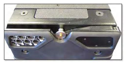
One issue with previous Martin Audio rigging system was the difficulty experienced flicking the rear linking bar out of its parked position. This problem has been solved with the addition or a protruding tongue at the base of the bar where it pivots. This can easily be used to rotate the bar out of its slot once the securing pin has been removed.
