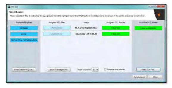
You can see that the optimisation contained within the file called "6 box test" appears in the Available D2.1 presets list on the right. It is also already showing in the Assigned D2.1 Presets for both of the left and right arrays in our system.
