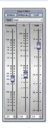
This shows all properties of the selected band. At the top you will see some text indicating which zone and which band the properties apply to. Below this are three buttons;-
