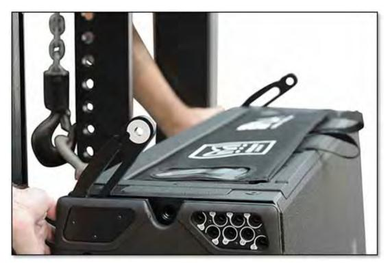
Align the holes in the rear bracket with the corresponding holes in the flying grid and pin them in place;-
