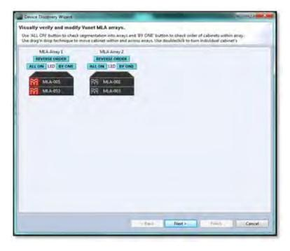
If you have more than one array the first step is to use the 'ALL ON' button which will illuminate all the LED badges on the array to check that the Vu-Net arrays match the physical deployment. If there are any errors the cabinets can be dragged and dropped to the correct positions or array. If you only have one array it is still worth flashing all LED's to see the look on the faces of the lighting technicians when they see LED lighting over which they have no control...
