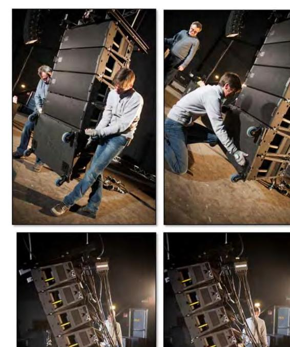
When you have connected the final Compact, connect the last Ceeform connectors to all remaining cabinets and the last link then the final U-Net cable that goes back up to the array loom checking for U-Net connectivity both on Port 2 of the final cabinet and on the Merlin.
