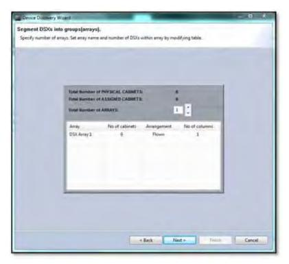
By default the 'Arrangement' will be displayed as 'Flown' therefore the 'No of columns' field will show 1. If you click on 'Flown' it will toggle to 'Ground Stacked' and if this is how your subs are deployed you can select the number of columns to reflect in Vu-Net exactly how they are positioned;-
