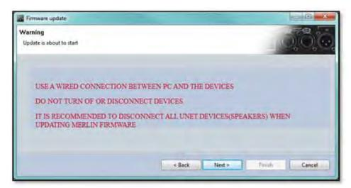
Click Next and the upgrade will start. A progress window will appear showing the processes in the upgrade taking place. The system tackles one device at a time, placing it into Boot Mode, uploading the firmware and rebooting the device back into an operating mode;-
