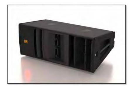
The MLD is the accompanying downfill enclosure to complement the MLA. It is designed primarily to be used at the bottom of an array using either a single MLD or a pair. Display 2.1 does not support any more than two MLD in an array. As a downfill box the dispersion is optimised for a wider coverage so the MLD has a horizontal coverage of 120° compared to MLA's 90°, and a vertical coverage of 20° compared to MLA's 7.5.
