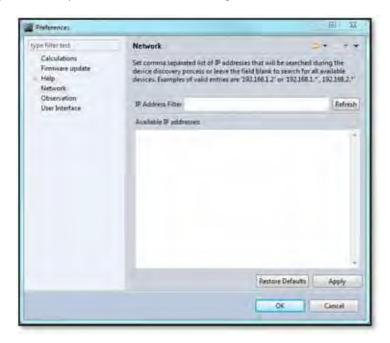
Running the application off line will display a blank window as shown. When you have one or more (usually at least two for MLA and MLA Compact systems) Merlins connected their unique IP address will appear listed in the bottom 'Available IP addresses'. You can set an IP address Filter in the smaller window which will search only for IP addresses within the range of values between the two entered which should be separated with a comma;-
