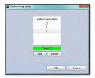
We want our top zone to consist of five MLA to click on the 10 shown in the top array and type "5". The quantity of cabinets is no longer 12 so the total is flagged red;-
