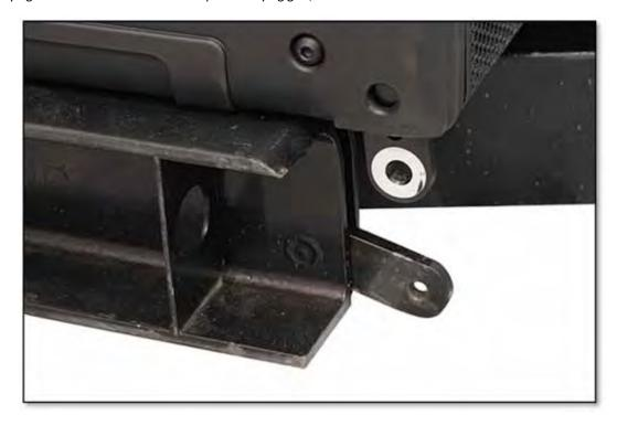
When the holes are aligned the cabinet can be pinned in place. It may help align the holes by lifting the rear of the MLA slightly.
