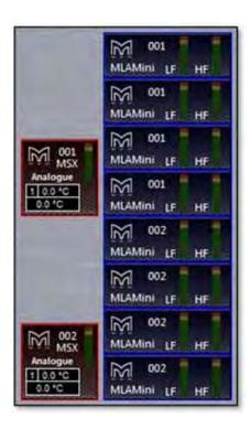
By default, MSX are assigned to zone 1 and all MLA Mini to zone 2. Reassigning zones is extremely simple. In our example we will keep the MSX assigned to zone 1, the top four MLA Mini to zone 2, the next two to zone 3 and the final two to zone 4. First click on the Zone 1 label;-
