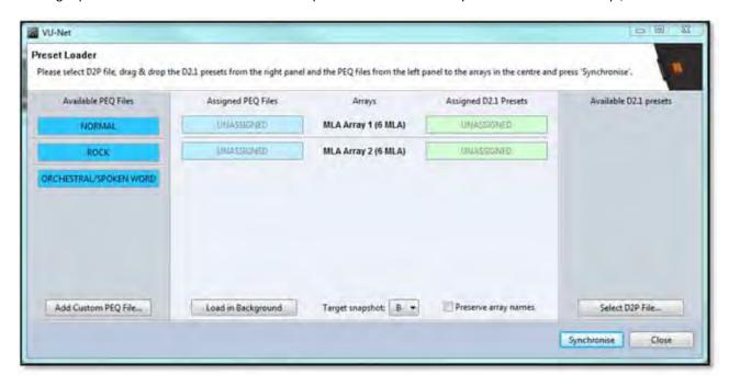
There are a number of options available but particularly when loading the first preset into an array the first step should always be to click on 'Select D2P File' to navigate to wherever you have saved the D2P file saved when you did your Display 2.1 optimisation (See Display Chapter for details);-
