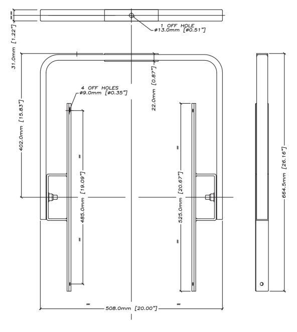
SUPPLIED HARDWARE:4 OFF M8x40mm CAP HEAD SOCKET SCREWS 2 OFF M12 'STAR' HANDWHEELS
