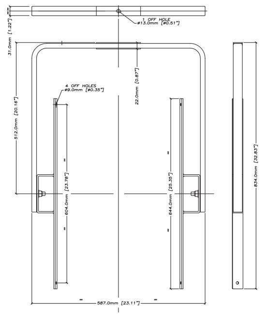
SUPPLIED HARDWARE:4 OFF M8x40mm CAP HEAD SOCKET SCREWS 2 OFF M12 'STAR' HANDWHEELS
