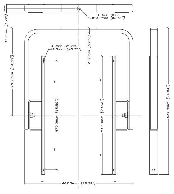
SUPPLIED HARDWARE:4 OFF M8×40mm CAP HEAD SOCKET SCREWS 2 OFF M12 'STAR' HANDWHEELS
