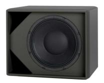
The Martin Audio Beatline I 12 is a direct radiating sub-bass in an ultra-compact heavily braced, vented enclosure. It features a very efficient I 2" (300mm) long-throw bass driver with a high power 3" (75mm) voice coil and generously sized low frequency ports for low noise, high power operation.
