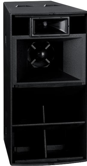
The Blackline H3T<sup>+</sup> is a very high performance, all-horn, three-way system in a single, wide-bandwidth package. New drivers have been developed for improved performance in all bands. The Hybrid® low frequency section comprises a horn-loaded 15" (380mm)/4" (100mm) voice coil driver that is reflex loaded to extend the LF output to below the natural horn cut-off point. The new LF driver features a water resistant cone and triple roll surround for increased excursion.
