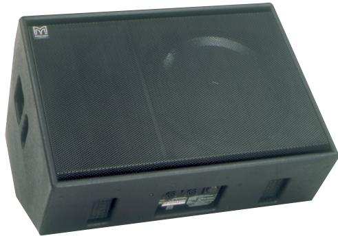
The Martin Audio LE700A is designed to overcome many of the problems associated with normal stage monitor systems, by utilising differential dispersion horn techniques to define a constant sound pressure level area in which the artist may move. In this area the frequency response and tonal characteristics remain unchanged.
