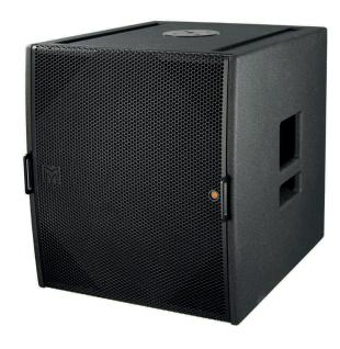
The PSX is a companion self-powered subwoofer for the DD6, XD12 and XD15 full-range loudspeaker systems. Featuring a powerful 15" (380mm) /4" (100mm) voice coil, long-excursion driver in a very compact reflex-ported enclosure, it houses two channels of Class D amplification — one channel for itself and one channel to power an XD12, an XD15, or up to three DD6's.
