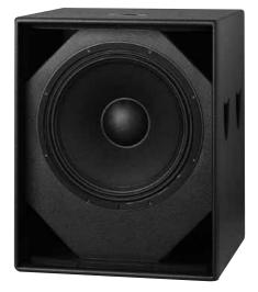
The compact Blackline \$18 sub-bass system has been designed to be used with Blackline \$12 and \$15 full-range systems to extend and increase the total low frequency output power. The \$18 provides good mid-bass punch with extended sub-bass output from a direct radiating 18" (460mm) driver with a 4" (100mm) high temperature voice coil.
