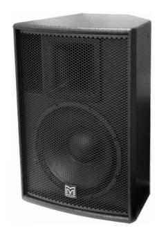
The Blackline  $X12^+$  is a high-power, high-output, two-way system equally suited to portable live sound applications and fixed installations. It features a high-specification  $12^{\circ}$  (300mm) low frequency drive unit and a  $1^{\circ}$  (25mm) exit compression driver mounted on a user-rotatable  $80^{\circ} \times 50^{\circ}$  constant directivity horn.
