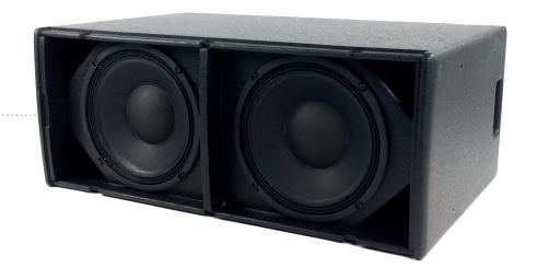
The X210 is a slimline dual-driver subwoofer designed for situations that call for a visually unobtrusive enclosure. It can be used singly, stacked or flown via integral M10 inserts and its ultra-compact size makes it ideal for applications where space is limited. It features dual 10" (250mm)/2" (50mm) voice coil drivers and generously sized low frequency ports for reduced air noise.
