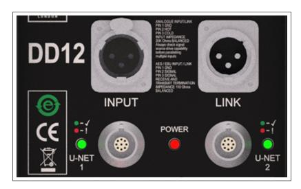
The connection panel is on the rear of the cabinet and features a female input XLR and a male Link XLR for balanced analogue or AES/EBU digital input signals. Input type is selected via Vu-Net software.
