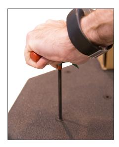
It is easier to fit a pole mount adaptor or scaffold clamp to the Universal Bracket before attaching it to the cabinet. Once this is complete, place the bracket in position and screw into place using the  $M8 \times 35$  mm screws supplied with the bracket. Ensure these are fully tightened.
