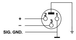
Figure 3. XLR input connector pin-out
