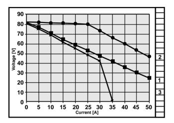
Figure 13. Current-voltage characteristic of different power supply topologies.
