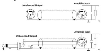
Figure 7. Unbalanced line connection
