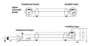
Figure 8. Balanced line with unbalanced equipment.
