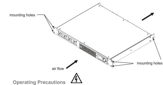
Make sure the AC mains voltage is correct and is the same as that printed on the rear of the amplifier. Damage caused by connecting the amplifier to improper AC voltage is not covered by the warranty. Make sure the power switch is off before making any input or output connections.
