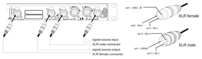
The figure below shows the connection of analog input for balanced and unbalanced line. You can use either configuration, but you must consider that unbalanced long lines can introduce noise in the audio system.
