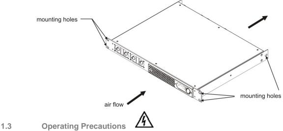
Make sure the AC mains voltage is correct and is the same as that printed on the rear of the amplifier. Damage caused by connecting the amplifier to improper AC voltage is not covered by the warranty. Make sure the power switch is off before making any input or output connections.
