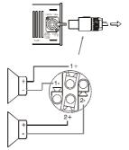
Channel A and B into one Speakon (Stereo and Bi-amp)
