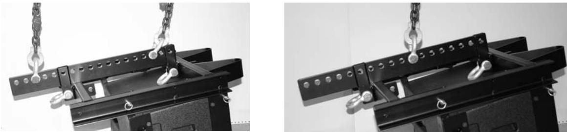
To attach the lifting bar, remove the two shackles from the pick-up lugs on the grid and attach the lifting bar to the lugs using the same shackles.
