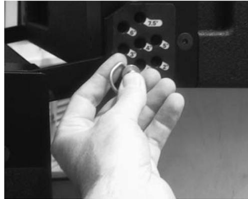
Position the next box face down on the floor beneath the rear of the grid. Lower the grid to align the rear of the flown box with the box on the ground. Remove the quick release pins from their storage locations and fold out the rear splay arms.
