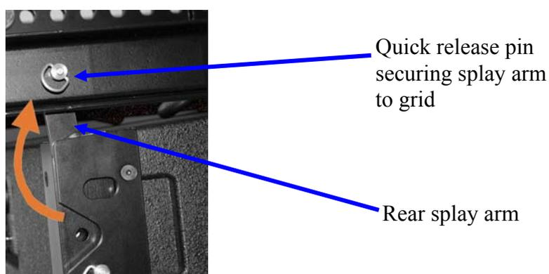
To attach the cabinet rear, remove the rear quick release pins and swing out each of the rear splay arms from its transit position up into the receptor at the rear of the grid.
