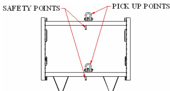
The standard grid is designed to fly an array of up to 16 W8LM enclosures with a 7:1 safety factor. Please use the ViewPoint™ array optimisation program to check that a particular array configuration maintains the 7:1 safety factor.
