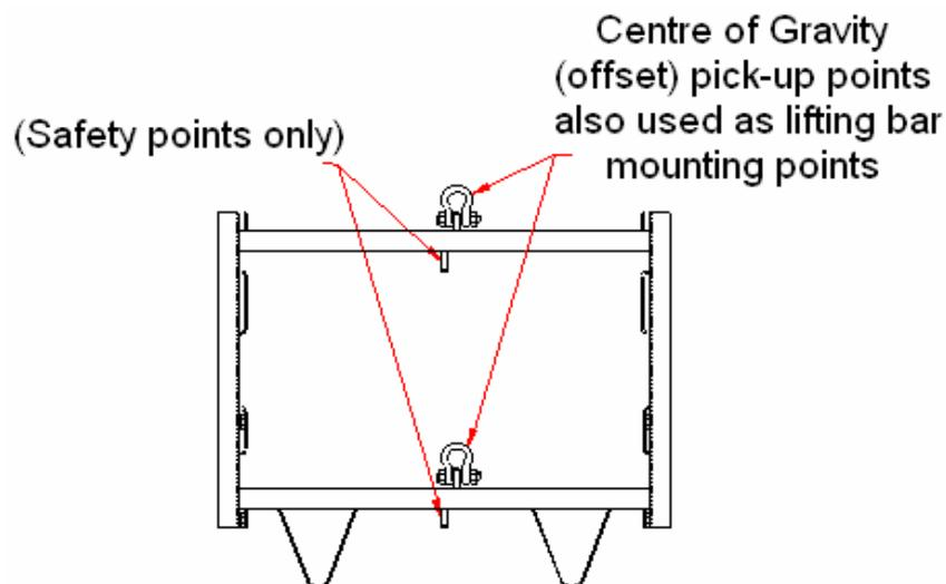
The lifting bar also has a number of holes along its length to facilitate single-point suspension using a single motor hoist. The bar can be attached as shown or rotated through 180° so that it protrudes from the front of the grid, in order to allow a greater degree of up tilt.
