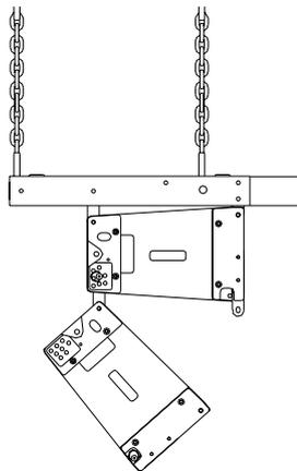
Lift the whole assembly until the lower cabinet clears the floor and is free to swing.
