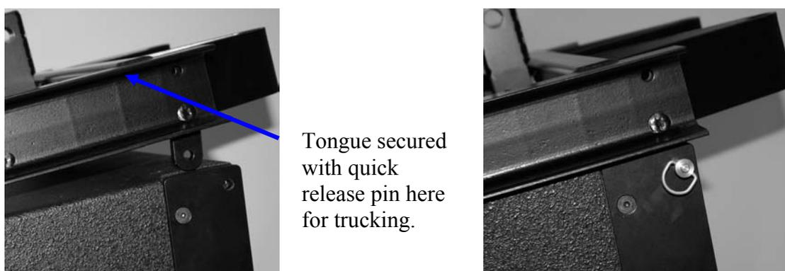
To attach the cabinet front, locate the grid tongues within the front brackets of the first box. Secure the tongues in position with the same quick release pins.
