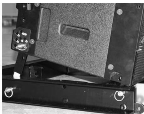
iv) Attach the ground stack bars into the rear receptors of the grid using the quick release pins that were removed from the front of the grid. Swing these bars up into the rear brackets of the cabinet and fix with quick release pins at the desired splay angle. (Use the two pins that are fitted to the additional pair of small attachment bars which are mounted to the sides of the grid)
