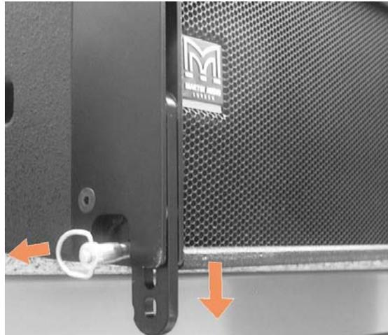
Lift the front of the hanging cabinet using the handles on the side and locate the front tongues within its front rigging assembly. Secure the tongues in position with the quick release pins.
