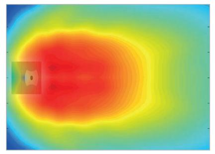
• XE500 SPL @ 6.3kHz over a 3 x 4m plane at head height Each contour represents 0.2dB change; yellow is -6dB
