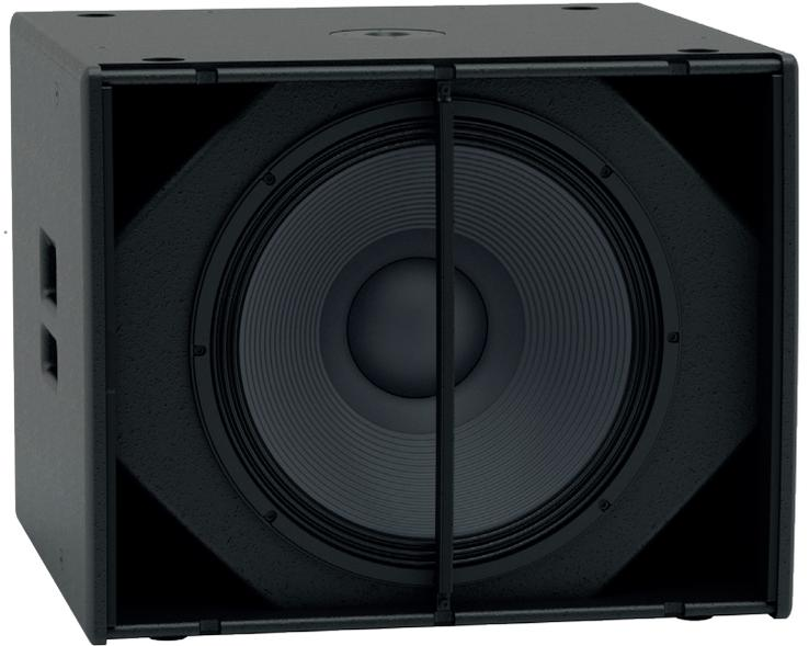
B118X extends the low frequency operating range of the combined system down to 42Hz and can be used singly, stacked in omni or cardioid mode, or flown via integral M10 insets. It features a long-excursion 18" (460mm)/4" (100 mm) voice coil driver in a compact enclosure that has four reflex ports with a large frontal area to reduce turbulent air noise at very high levels.
