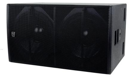
The B218X is a dual-driver, high performance subwoofer for use with full-range loudspeakers. With an operating range of 42Hz-200Hz + 3dB, it produces high output levels with low distortion and can be used singly or stacked horizontally. It features dual 18" (460mm)/4" (100mm) voice coil, long-excursion drivers in a reflex enclosure with eight large ports that reduce air turbulence at high output levels.
