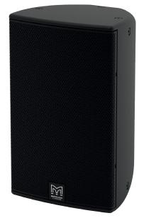
The visually distinctive composite enclosure can be used in either horizontal (landscape) or vertical (portrait) orientation, with rotation of the driver easily accomplished by removing the screw-free, protective grille. The curved shape of the CDD10TX allows it to be surface-mounted close to a wall via an optional wall bracket or suspended from a ceiling by eyebolts or a horizontal yoke option.
