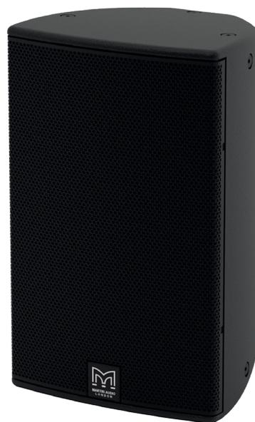
The CDD10 is a very compact two-way passive loudspeaker system which utilises a 10" (250mm) LF/1" (25mm) exit HF Coaxial Differential Dispersion driver. It is uniquely placed to meet the foreground requirements of music bars and clubs, as well as the varied architectural applications that require upfront sound levels from a very compact enclosure. Use with a SX118 or SX218 subwoofer will enable the CDD10 to operate as small dancefloor system that is remarkably powerful for its size.
