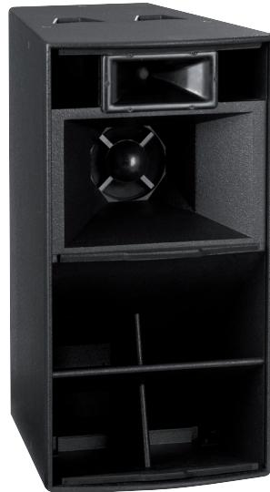
The Blackline H3<sup>+</sup> is a very high performance, all-horn, three-way system in a single wide-bandwidth package. New drivers have been developed for improved performance in all bands. The Hybrid® low frequency section comprises a horn-loaded 15" (380mm)/4" (100mm) voice coil driver that is reflex loaded to extend the LF output to below the natural horn cut-off point. The new LF driver features a water resistant cone and triple roll surround for increased excursion.
