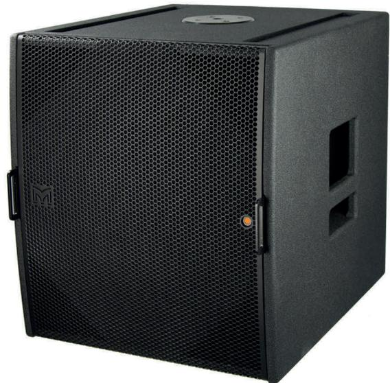
The PSX is a companion self-powered subwoofer for the DD6, XD12 and XD15 full-range loudspeaker systems. Featuring a powerful 15" (380mm) /4" (100mm) voice coil, long-excursion driver in a very compact reflex-ported enclosure, it houses two channels of Class D amplification — one channel for itself and one channel to power an XD12, an XD15, or up to three DD6's.
