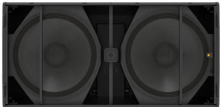
The SX218+ delivers very high output levels and superb transient performance with minimal distortion, making it ideal for the most demanding applications. With an operating range of 38 Hz–100 Hz  $\pm$  3 dB, it houses dual 18 in (460 mm) long-excursion drivers with 4 in (100 mm) voice coils, water-resistant cones and triple-roll surrounds. Each driver is rated to handle 1500 watts AES and has a magnet structure and suspension engineered for maximum linear excursion.
