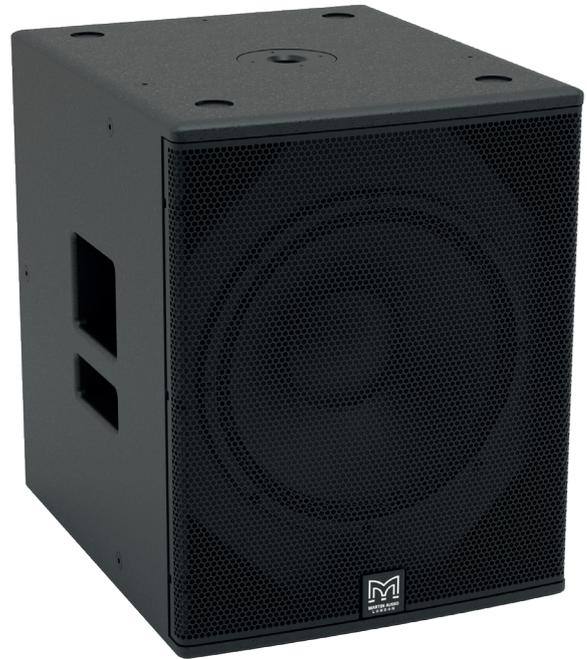
The X115 is a very compact subwoofer designed to augment the low frequency performance of BlacklineX Series full-range systems. It comprises a long excursion 15" (380mm)/3" (75mm) voice coil driver in a bass reflex enclosure and can be used singly, stacked or flown via integral M10 inserts. Four large ports contribute to a reduction in air noise at high output levels.
