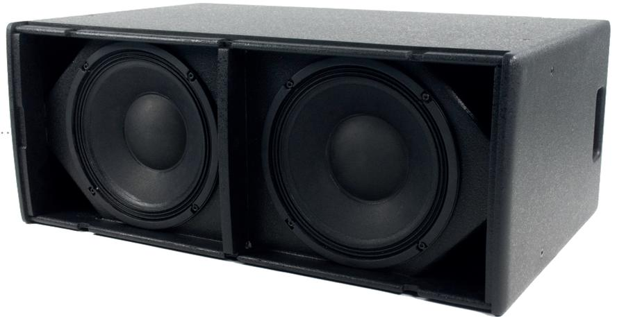
The X210 is a slimline dual-driver subwoofer designed for situations that call for a visually unobtrusive enclosure. It can be used singly, stacked or flown via integral M10 inserts and its ultra-compact size makes it ideal for applications where space is limited. It features dual 10" (250mm)/2" (50mm) voice coil drivers and generously sized low frequency ports for reduced air noise.
