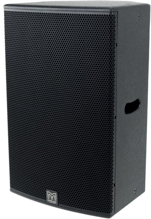
The high power Blackline XH15 provides improved performance over the Blackline X15 in a wide-bandwidth system and a compact and efficient package. Extended frequency response is provided by a 15" (380mm) LF driver and a 1.4" (35mm) exit compression driver mounted on a rotatable 80° x 50° constant directivity HF horn.
