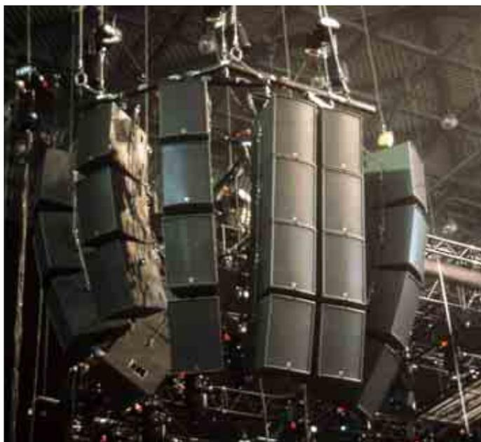
bleachers with bass projection provided by a combination of flown W8CS run as mid-bass and floor-stacked WSX folded horn subwoofers.
