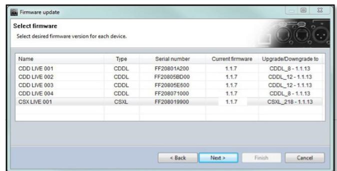
You can see the current firmware installed in each cabinet which is version 1.1.7 and the new version which is 1.1.13.
