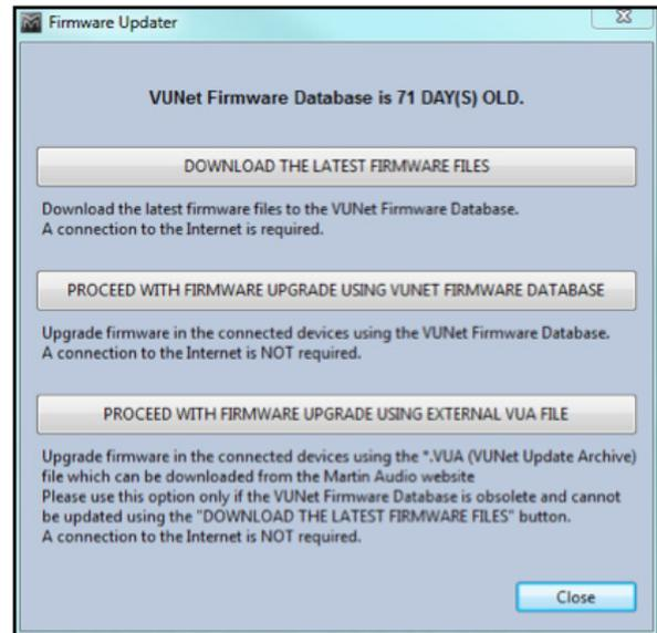
4. At the top of the window we can see how old the firmware database is. Select 'DOWNLOAD THE LATEST FIRMWARE FILES'. This will connect to the Firmware Server over the web and will download the latest firmware files including the new version for the CDD Live range. You will see the following window while the download is in progress;-
