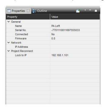
Having a well-managed static system also means that troubleshooting a faulty device is much easier. Replacing a faulty amplifier that has the correct settings for the system is easy to achieve with a static setup as the virtual device can be synchronised to a physical device that share the same IP address.
