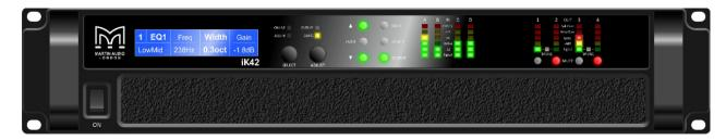
To set a static address for iKON, select *Utility* on the amplifier's front panel then push the up arrow twice. Here you can toggle between *Auto* and *Static* modes using the right encoder.
