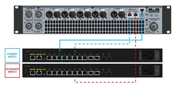
Just like iKON's ethernet control, the Dante card has the option to use automatic or static IP addressing. If a DHCP server is connected to the primary port of the rack, then both control and Dante primary ports will receive IP addresses from the server. If no DHCP server is present, a link-local address will be used.
