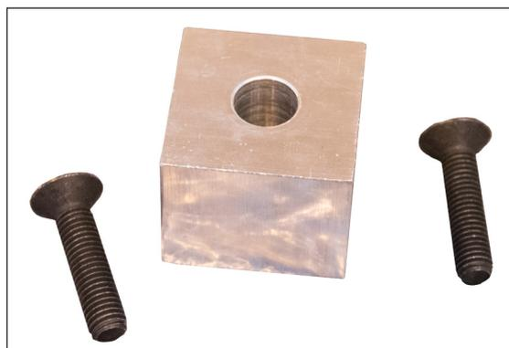
**IMPORTANT:** It is essential that the M8 x 35 screws are used to fit the bracket. Do not use the existing screws in the cabinet M8 inserts, which are too short, and are not rated for use with flown systems. A flown DD12 using these screws to fix the bracket will NOT be safe.
