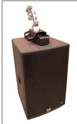
The ASF20046 Universal Bracket allows the DD12 to be mounted in a number of ways. It can be fitted to with the top, bottom or side of the cabinet, and offers a single 13 mm (1/2") fixing point which can be used to secure the cabinet to any standard 35 mm speaker stand using a pole mount adaptor (Part No. ASF20045) or a scaffold clamp.
