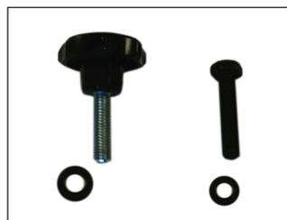
Either the handwheel or the bolt may be used; the former is preferable if the cabinet is likely to require subsequent readjustment; use the bolt if the cabinet angle should not be altered. Note that both the handwheel and M8 bolt are high tensile steel, rated to take the weight of the cabinet. Do not use other fixings under any circumstances, as this may result in the assembly not meeting its safety rating.
