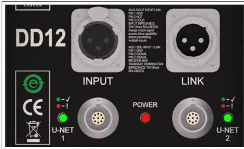
The connection panel is on the rear of the cabinet and features a female input XLR and a male Link XLR for balanced analogue or AES/EBU digital input signals. Input type is selected via Vu-Net software.
