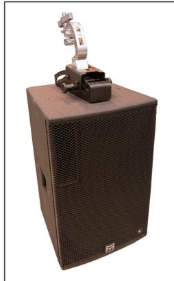
The ASF20046 Universal Bracket allows the DD12 to be mounted in a number of ways. It can be fitted to with the top, bottom or side of the cabinet, and offers a single 13 mm (1/2") fixing point which can be used to secure the cabinet to any standard 35 mm speaker stand using a pole mount adaptor (Part No. ASF20045) or a scaffold clamp.
