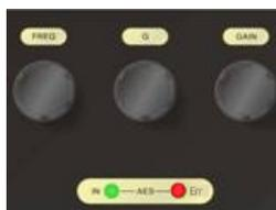
The two status LEDs indicate that **AES** inputs have been selected and **Error**.
