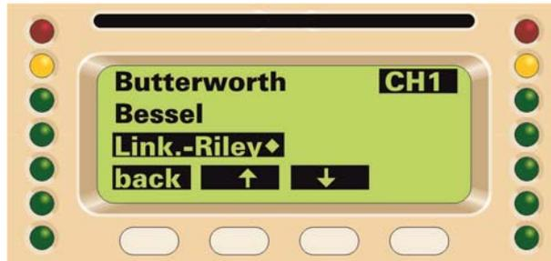
Set Shape=Linkwitz-Riley (You could also experiment with shape=FIR)
