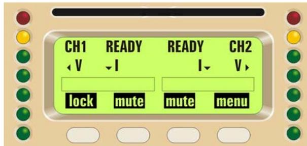
The LED bars can function as output voltage or output current meters; in the first case the LCD meters function as output current meters, vice versa in the second case. The first green LED at the bottom of the LED bar when illuminated indicates the presence of input audio signal above -60 dBV on the corresponding channel.
