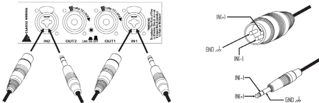
The figure below shows the connection of analog input for balanced and unbalanced line. You can use either configuration, but you must consider that unbalanced long lines can introduce noise in the audio system.
