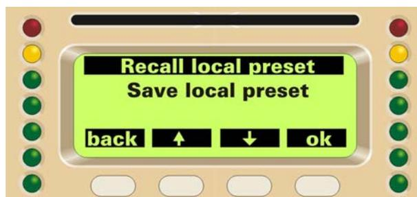
You can select the desired option by pushing up or down button and "ok" to activate it. The option "Recall local preset" does not appear if the smartcard is blank.
