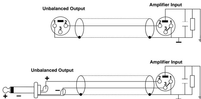
Figure 7. Unbalanced line connection
