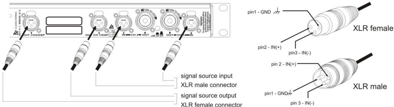
The figure below shows the connection of analog input for balanced and unbalanced line. You can use either configuration, but you must consider that unbalanced long lines can introduce noise in the audio system.
