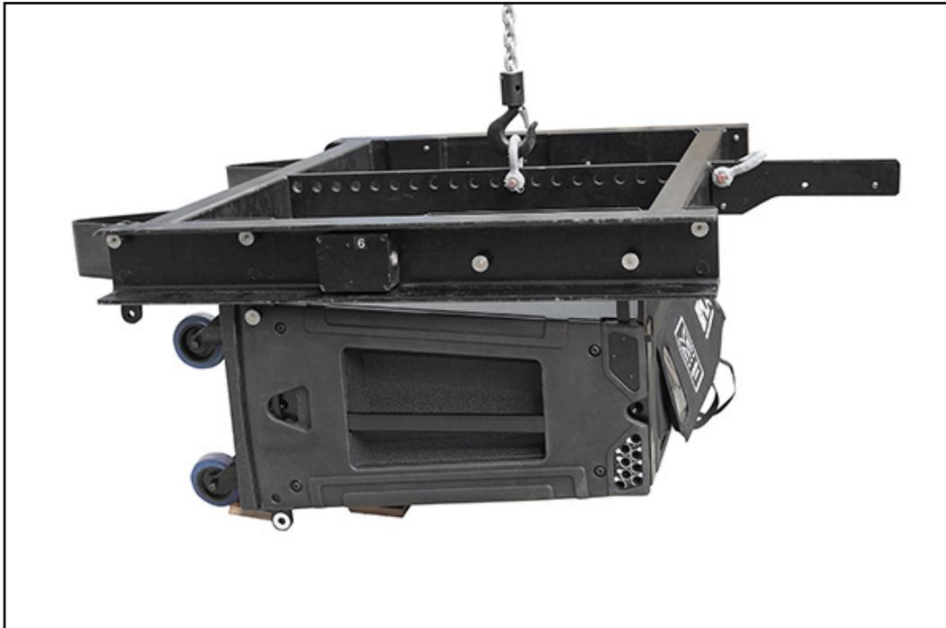
In this position it is relatively easy to connect the front rigging pins to the grid. The array can then be flown and the rest of the array rigged in exactly the same way as before;-
