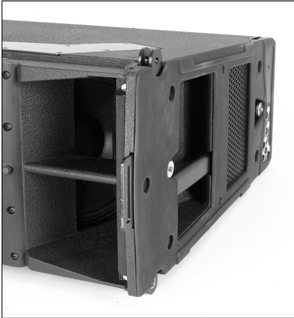
The slot-loading allows the twin LF drivers to be optimally spaced within the enclosure. The double-source arrangement significantly improves the directivity control of the LF section maintaining the 100 degree system beamwidth down to 250Hz and reducing mid-bass output at the sides and rear of the array. The LF drivers themselves are very high excursion with vented poles to reduce power compression and virtually eliminate turbulent air noise.
