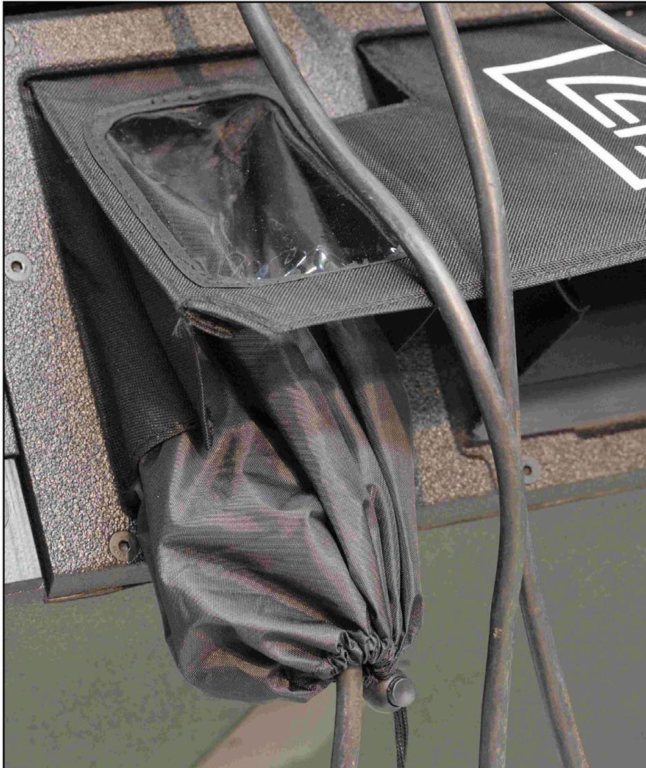
The final step is to tidy the cables to keep the loom neat, particularly any spare Ceeform cables if your array is smaller than 12 boxes. Over-hanging cables should be neatly coiled and taped behind the array so they are invisible to the audience.
