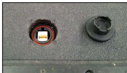
Note that early MLX did not have the cabinet mounted RJ45 port. All MLX should have been modified to fit the socket but if this hasn't happened it will be necessary to remove the amplifier module to access the RJ45 port on the module itself.
