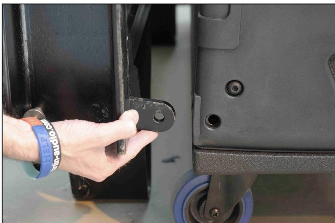
It is important to make sure that this is done simultaneously on both sides, it is almost impossible to connect into the MLA if it is not square to the grid. The front rigging bracket on the MLA will be pushed out so it protrudes from the bottom of the cabinet. When the bar is fully inserted into the cabinet rigging point so that the holes line up, insert the pin that you removed from the cabinet;-
