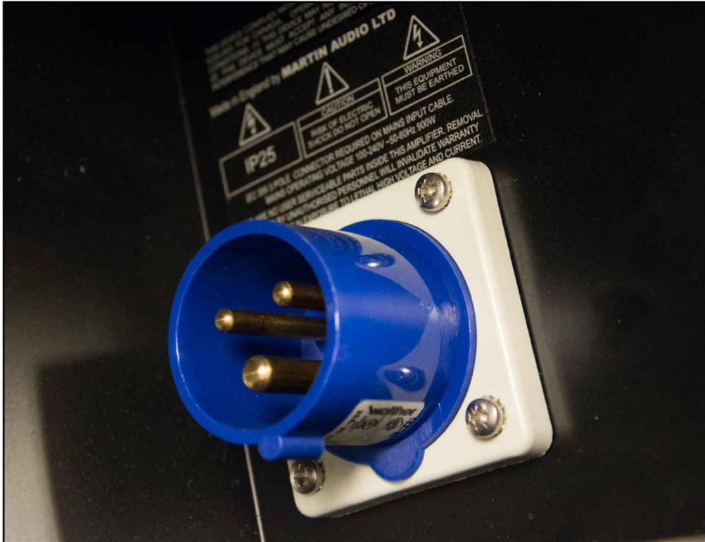
The MLX has a universal PSU suitable for direct connection to virtually any mains voltage anywhere in the world. It is supplied fitted with a 16A Ceeform single phase mains inlet. If you are not using the Martin Audio MLA distribution system a matching Ceeform 16A female outlet connector must be used. For outdoor use this should be rated at IP67, this is to ensure safe operating when any connectors are disconnected in damp conditions.
