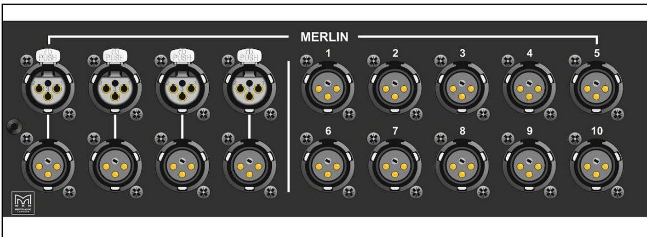
As well as all ten outputs being available there is a parallel connection to all four inputs to make it easy to daisy-chain audio feeds between racks if necessary.
