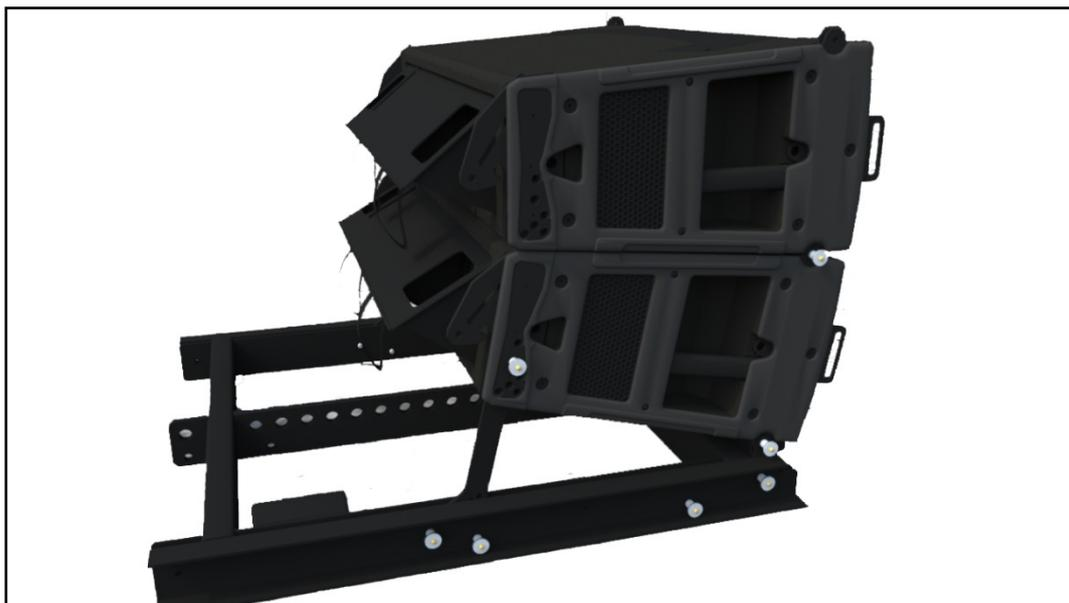
Raise the back of the cabinet and link the cabinets at the angle shown in your Display project;-
