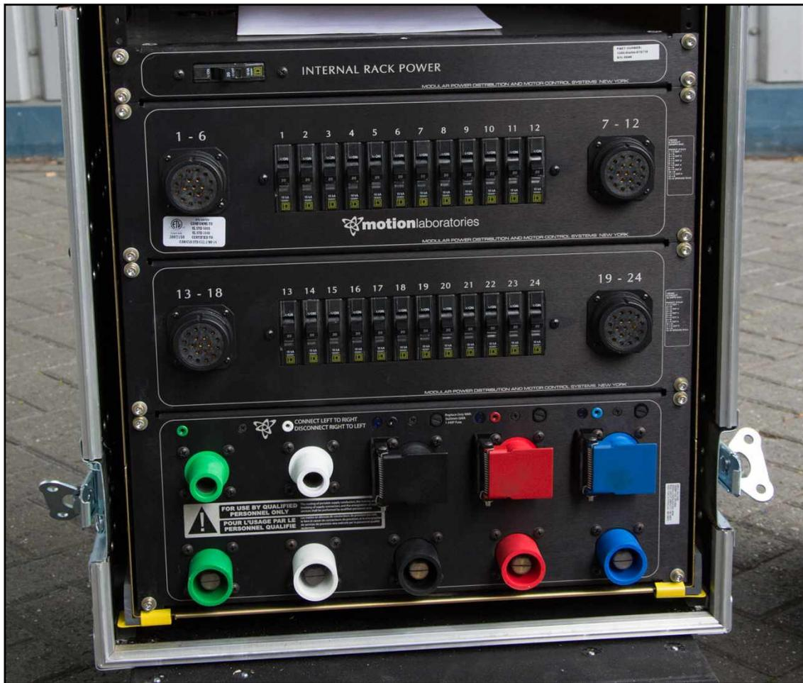
For territories with lower mains voltage supplies below 200V AC, a high current mains distro is available. All MLA products have switch mode power supplies so they can be used at any mains voltage anywhere in the world however the lower the mains voltage the higher the current draw for consistent power output therefore the distro is required to cater for a much higher current draw.
