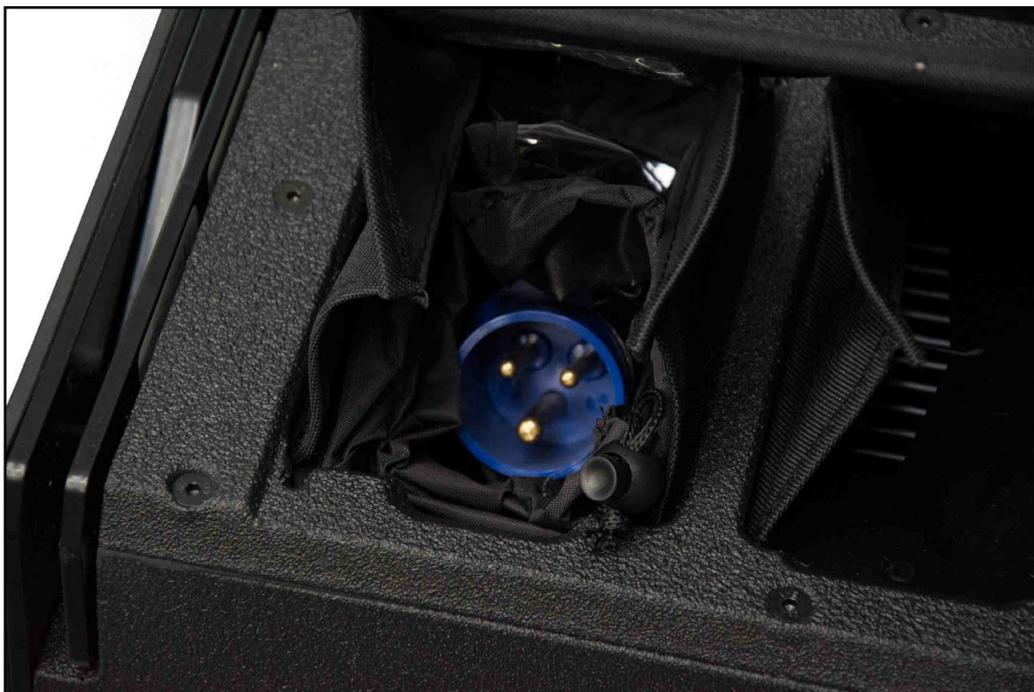
The MLA Compact has a universal PSU suitable for direct connection to virtually any mains voltage anywhere in the world. If you are not using the Martin Audio MLA distribution system a matching Ceeform 16A female outlet connector must be used. For outdoor use this should be rated at IP67, this is to ensure safe operating when any connectors are disconnected in damp conditions.
