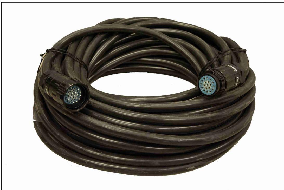
**ASF12002** is a 30m 18-core multiway mains cable terminated with Tourmate 19-pin connectors, one male, one female. Tourmate is based on the popular Socapex pattern but is rated at IP67 when mated so is suitable for use outdoors in all weather. The cable has 18 cores each 2.5mm<sup>2</sup> and has a tough, flexible outer sheath. Other lengths are available to special order. The Tourmate is used to connect a Master or Slave rack to an array.
