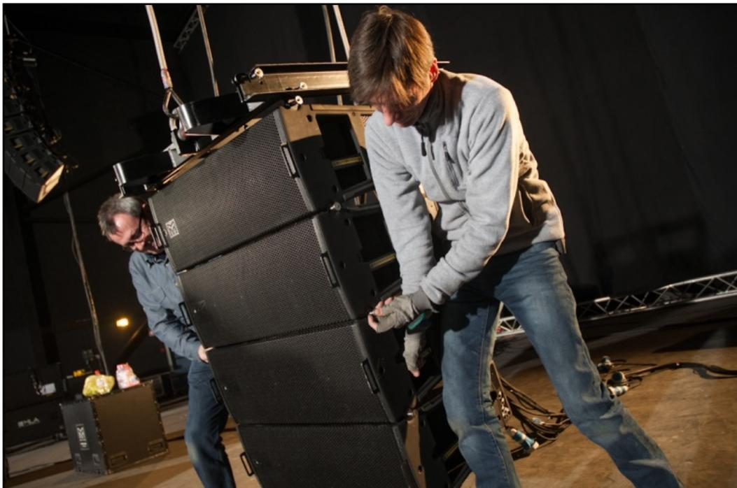
Remove the wheelboard then connect power to cabinets 2 and 3 but NOT 4, as we have mentioned, the Ceeform on the lower cabinet will make it difficult to rig the next pair of Compact. Connect link cables from cabinet 2 to 3 and 3 to 4, check that they power up correctly and that you get U-Net LEDs illuminating on all powered cabinets.
