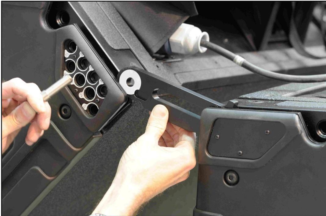
Check which hole needs to be connected from the optimisation that you did with Display 2.1 and connect the rear brackets with the flying pins;-
