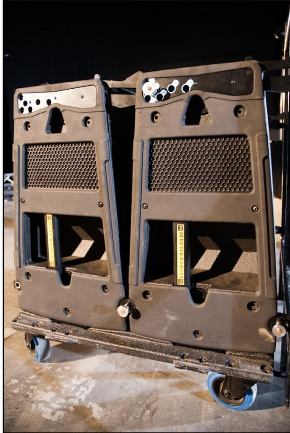
The Compact will have to be lined up completely square to the grid or it will be impossible to line up the holes in the grid and cabinet bracket. Connect the first cabinet to the flying frame, first with the front bracket;-
