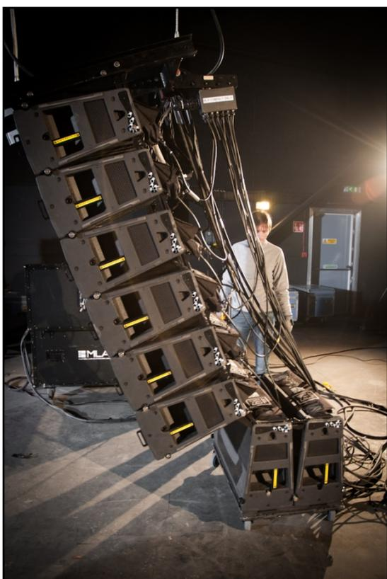
When you have connected the final Compact, connect the last Ceeform connectors to all remaining cabinets and the last link then the final U-Net cable that goes back up to the array loom checking for U-Net connectivity both on Port 2 of the final cabinet and on the Merlin.
