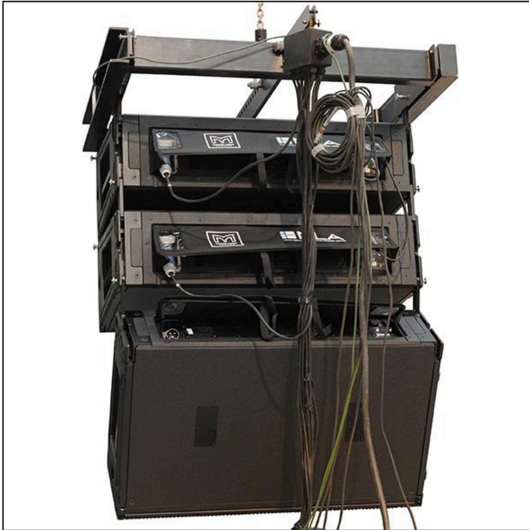
Connect power to the second cabinet (not the third) and check that you see the cabinet power up and U-Net LED's illuminate on both the first and second cabinets. Add another pair of link cables from the second and third cabinets.
