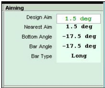
Rather than specifying which hole in the bar is shown the bar angle as the bar itself has a label with shows which holes to use to achieve the desired angle. Once again where there is a difference in the design aim to that which can be achieved with the ground stack bar the design aim is shown in red with the 'Use Nearest' option available. If clicked the design aim and array diagram will be updated;-
