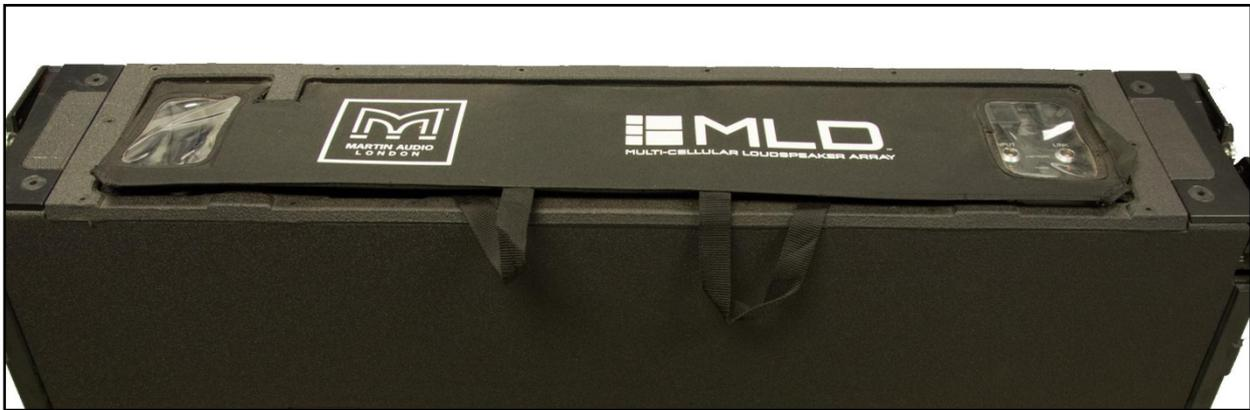
The cowl travels folded flat for ease of transportation. It is held in the operating position by two triangles of canvas mounted towards the middle of the cowl. These have straps attached and by pulling the straps the cowl pops up into position and is held in place with the two supporting triangles which connect to the inside of the cowl using Velcro. To fold the cowl flat, the straps are again used to pull the supporting triangles down left and right.
