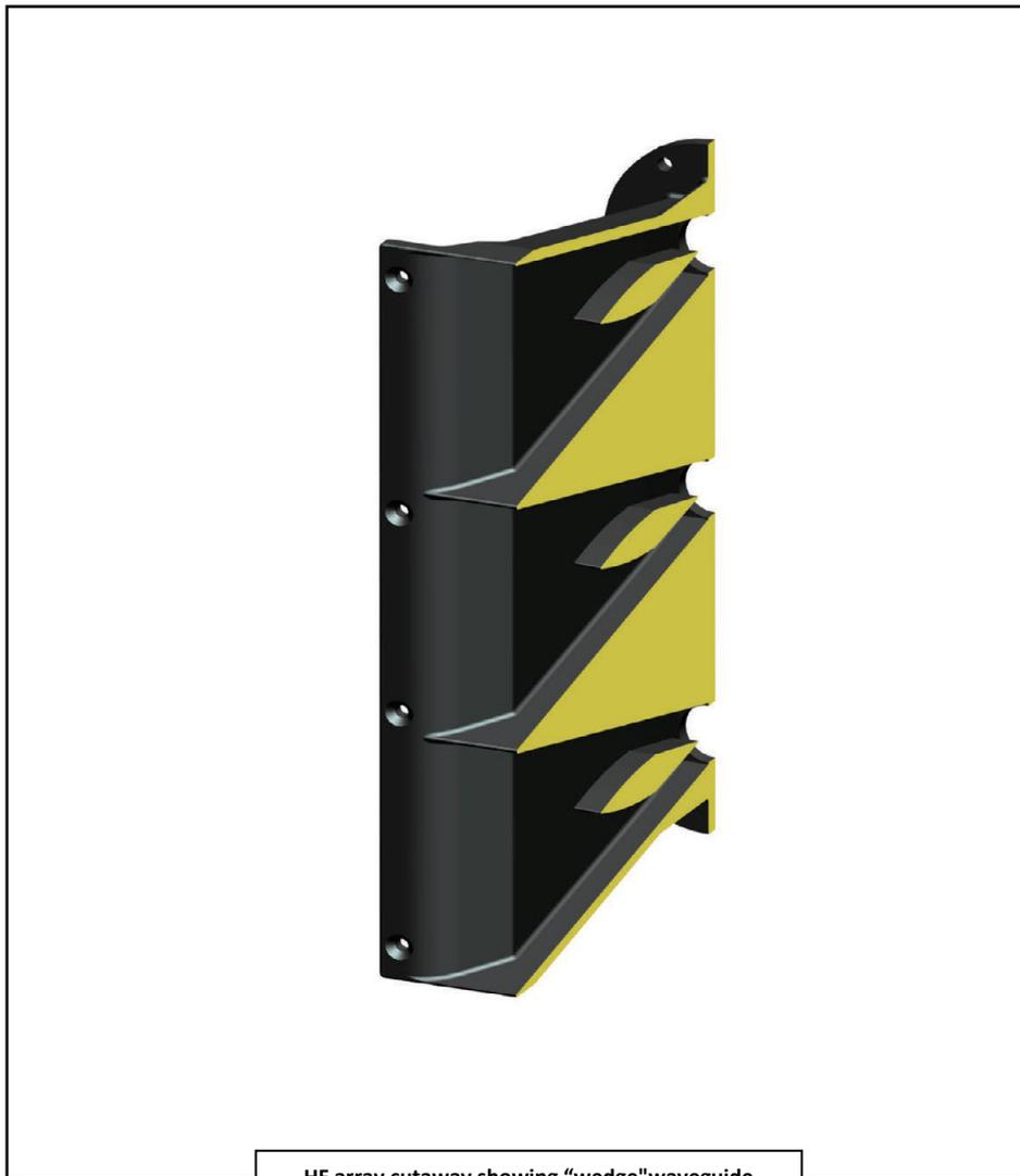
HF array cutaway showing "wedge" waveguide
