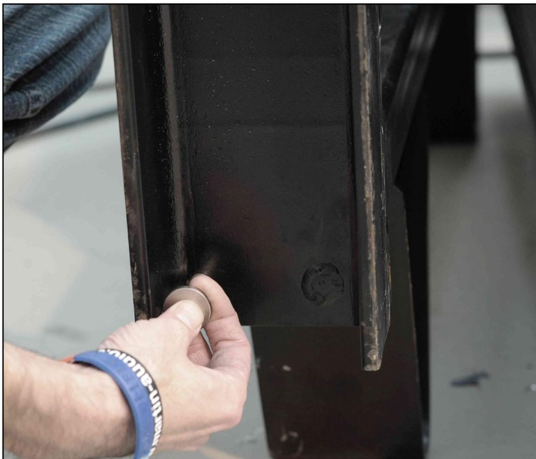
A short steel bar will swing down on each side. With one person at each side of the grid, remove the flying pin from the front centre stowing position on the MLA and carefully wheel the cabinet up to the grid, directing the metal bar into the top flying point of the cabinet;-
