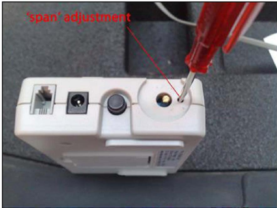
Carefully adjust the pot until the display matches the reference. Next lower the grid to around  $-30^{\circ}$  and  $-20^{\circ}$  checking each time that the reference and reader displays match. It may be necessary to re-adjust the zero measurement following calibrating the span, in which case check the span calibration again.
