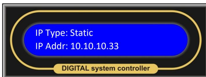
Three presses of the 'Back' button will return you to the main menu. Power cycle the Merlin and return to the Network Settings submenu to double check that the settings are correct.
