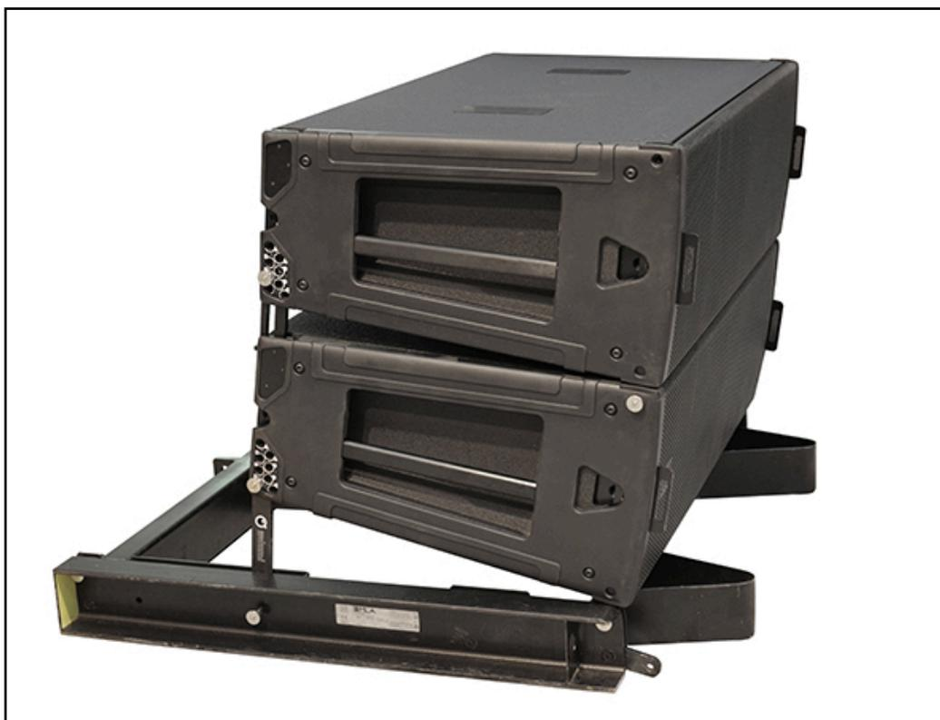
Unlike a flown array you are advised not to wire the array as it is built, the cabling is likely to get in the way and as the system is ground stacked it is usually very easy to access the connection points when you have finished building the stack;-
