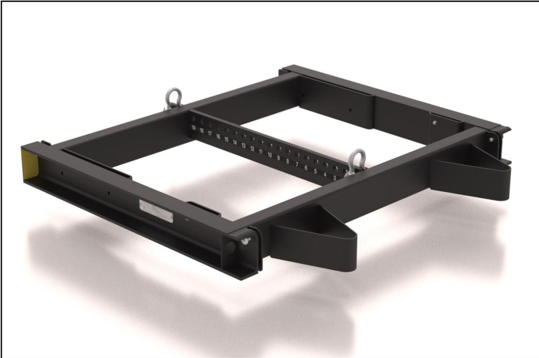
The MLA flying Grid is the principal system for deployment of MLA systems. When used with a two point suspension system it can be used to fly up to 24 MLA or 15 MLX or a maximum of 6 MLX with 12 MLA flown below in a combination array (note that this configuration requires two grids). The grid features a central spine which allows single point rigging of up to 10 MLA.
