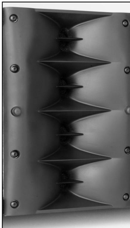
MLA Compact’s HF section utilises 4 × 0.7" (19mm) exit neodymium compression drivers which feed separate horns for true 100° horizontal constant directivity. In the vertical plane, MLA Compact makes significant advances over previous thinking by adopting new criteria for vertical wavefront curvature.
