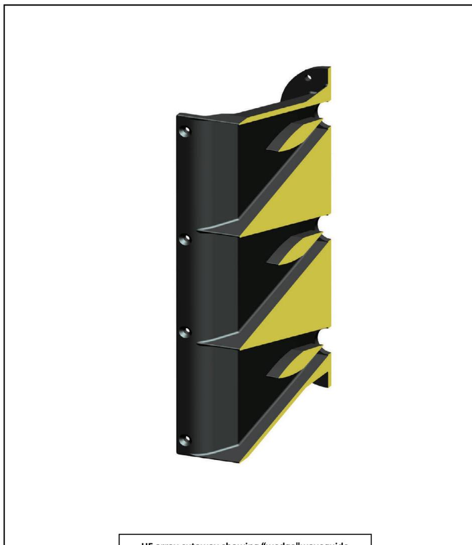
HF array cutaway showing "wedge" waveguide
