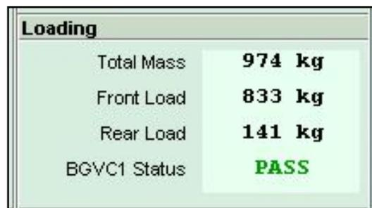
This shows the mass that each point will see, in this example 833Kg for the front point and 141Kg for the rear point.
