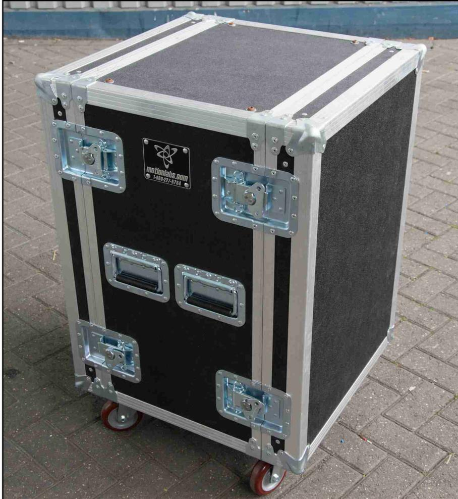
The low voltage rack case has remained unchanged since its introduction and is a 15U floating rack flightcase into which the mains distro is permanently built leaving a 4U space at the top for the Merlin and network products. It is constructed from black laminated ply and has always used natural, silver extrusions and fittings. It has front and rear lids both secured with four butterfly catches.
