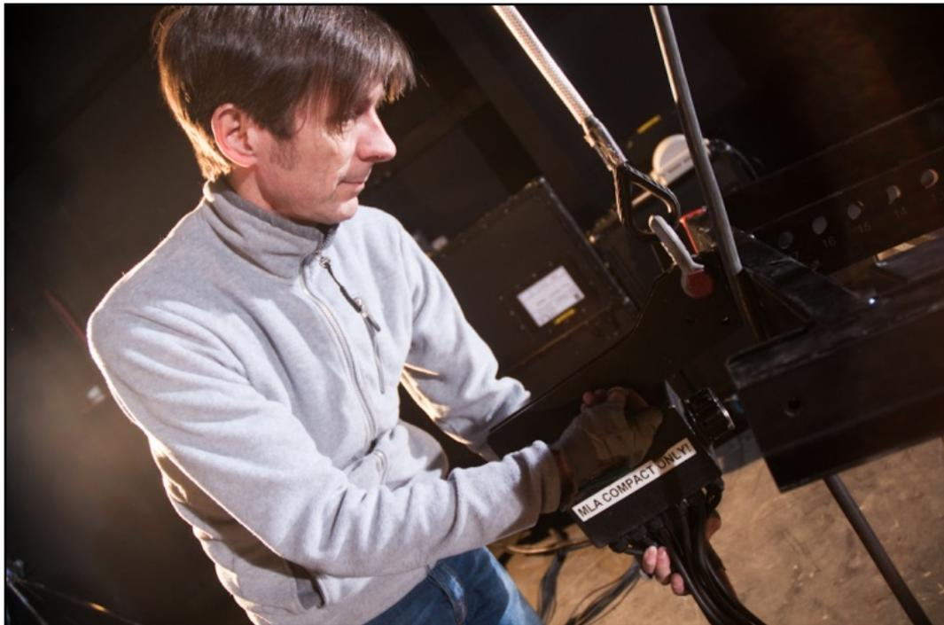
Connect the U-Net cable designated for the top cabinet to U-Net port 1 and the audio XLR cable to the XLR input on the first cabinet. Connect the Inclinometer cable to the sensor on the grid;-
