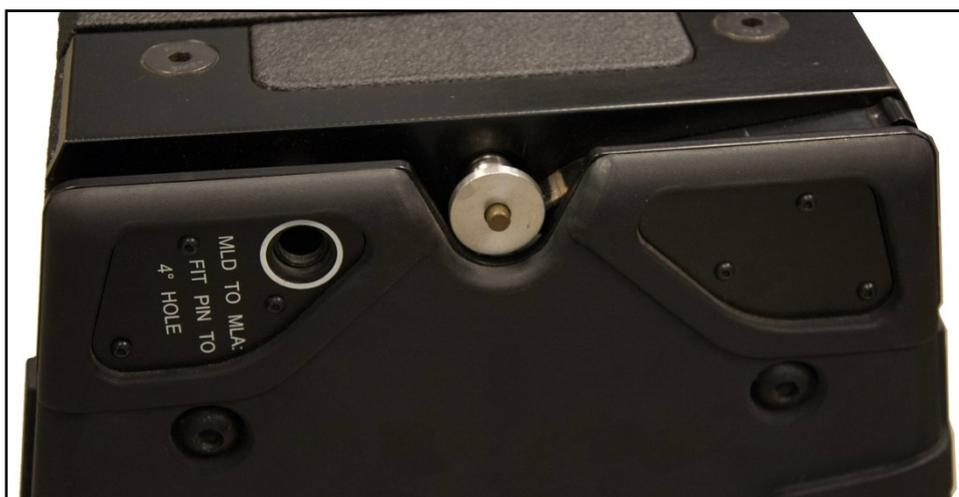
The rear bracket swings up as the MLA to join to an array but links to one position to give an angle of 13.75°. There is only a single hole in the bottom of the bracket to accommodate a second MLD in the array which will give a fixed angle between the two of 20°.
