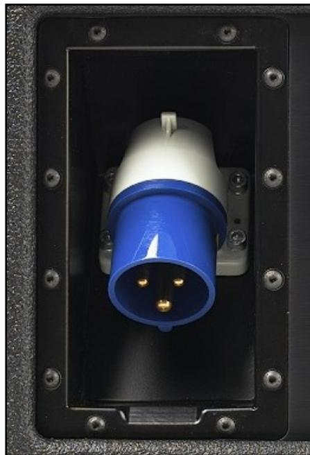
The MLA has a universal PSU suitable for direct connection to virtually any mains voltage anywhere in the world. If you are not using the Martin Audio MLA distribution system a matching Ceeform 16A female outlet connector must be used. For outdoor use this should be rated at IP67, this is to ensure safe operating when any connectors are disconnected in damp conditions.
