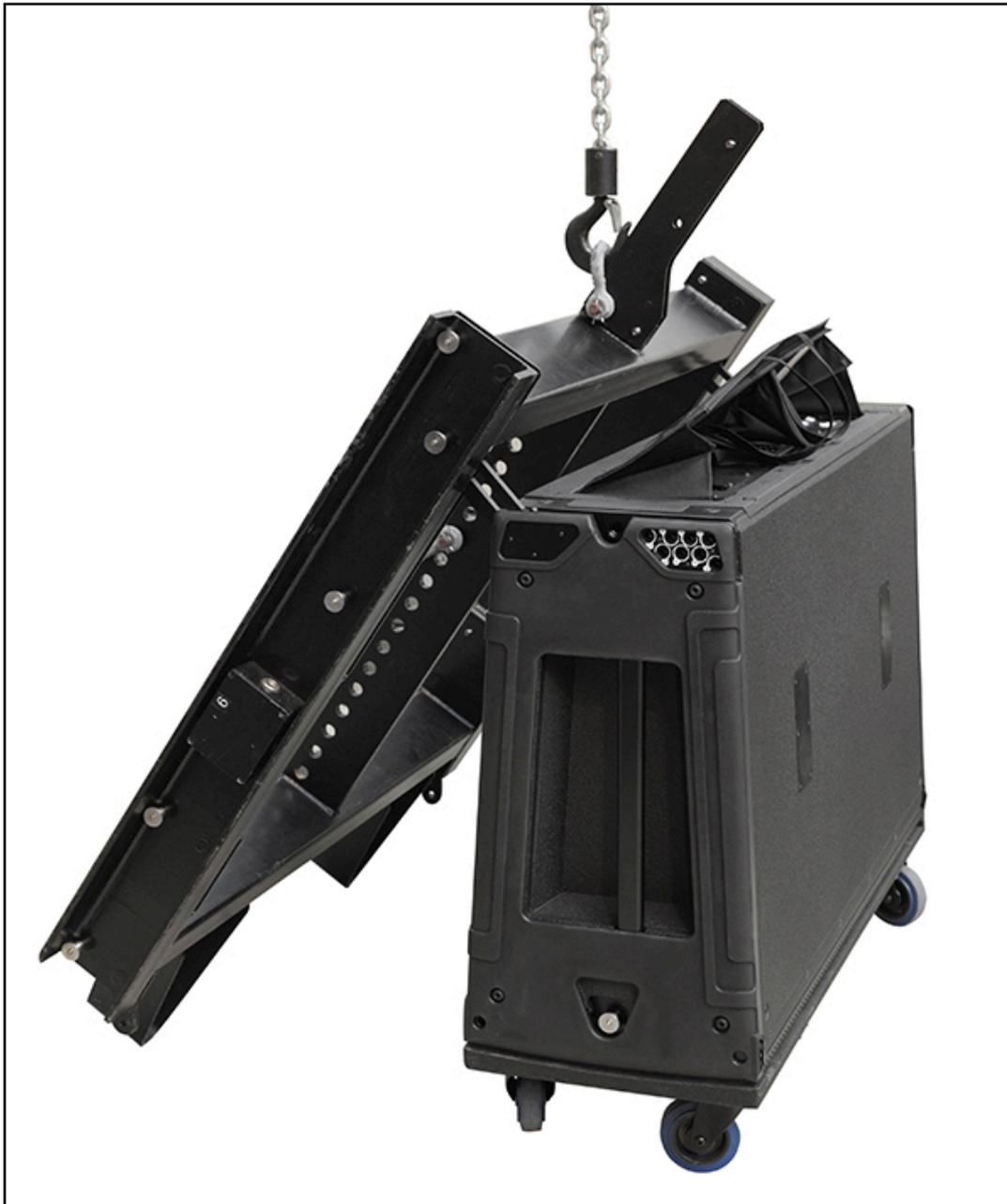
Connect the rear bracket to the holes at the back of the flying grid. As the cabinet is at the back of the grid it is impossible to line up the front rigging positions with the cabinet and grid vertical, it is also difficult to swing up the cabinet to the grid as the grid has little stability with no cabinets attached so it will move around making it awkward to fir the pins. The easiest option is to fly
