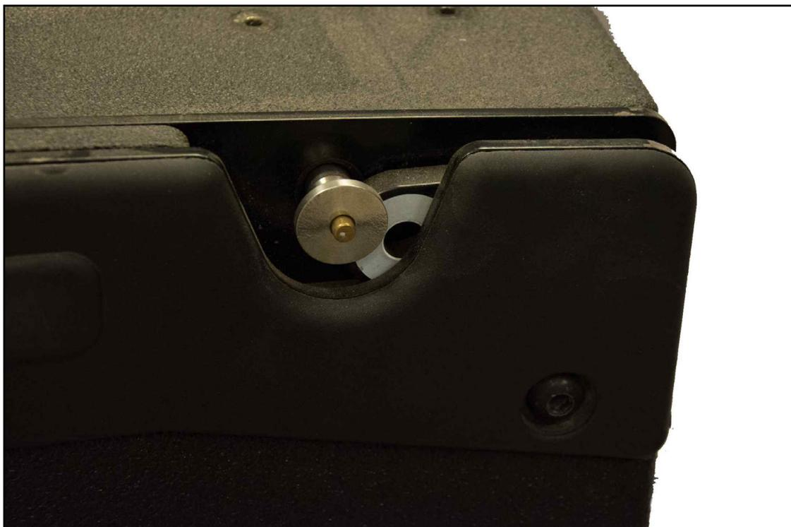
The rigging bar hinges up and is secured in its stored position with a flying pin.
