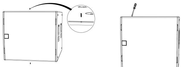
Remove the screws from the grille support on the side of the cabinet and remove the grille support.
