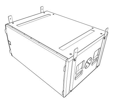
Fit the SX218FKIT flying kit to each cabinet. There are four steel brackets in each kit and these attach vertically, two on each side of the subwoofer. Remove all four M10 bolts in the inserts on the sides of the cabinet.
