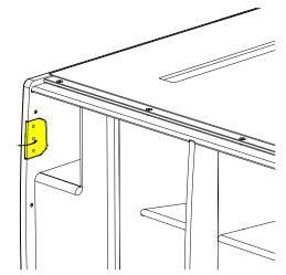
Screw the bracket back in place and repeat for the other three brackets.
