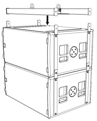
Join using the four M10 x 50 button head screws and washers supplied with the grid assembly. The sub can now be safely flow to the desired height.
