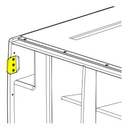
Replace the grill supports and fit the grille making sure the safety screws are replaced.
