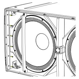
Remove the three screws from the bracket.
