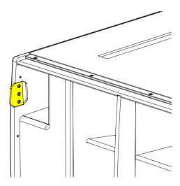
Replace the grill supports and fit the grille making sure the safety screws are replaced.
