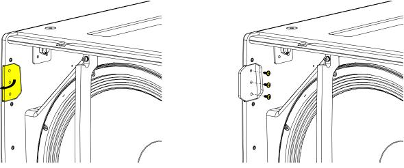
Replace the grill supports and fit the grille making sure the safety screws are replaced.
