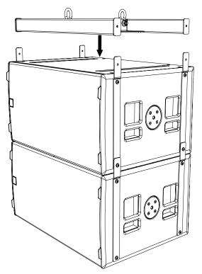
Join using the four M10 x 50 button head screws and washers supplied with the grid assembly. The sub can now be safely flow to the desired height.
