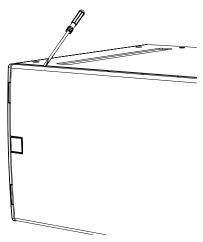
Remove the screws from the grille support on the side of the cabinet and remove the grille support.
