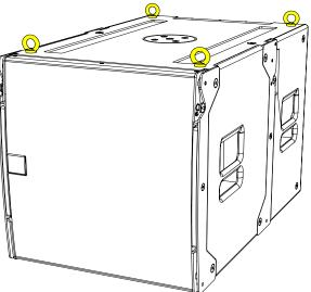
Eyebolts should be connected to a suitably rated fixing point such as a girder clamp or a heavy duty fixing such as a sleeve anchor or similar. They can be linked using suitably rated steel rope or chain and shackles.
