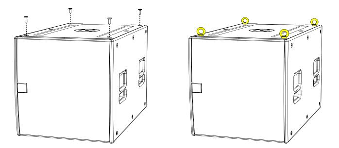
Eyebolts should be connected to a suitably rated fixing point such as a girder clamp or a heavy duty fixing such as a sleeve anchor or similar. They can be linked using suitably rated steel rope or chain and shackles.
