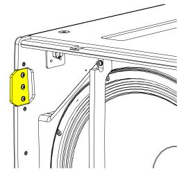
Replace the grill supports and fit the grille making sure the safety screws are replaced
