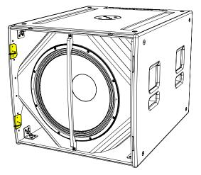
Screw the bracket back in place and repeat for the other three brackets.
