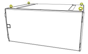
Remove the M10 counter-sunk screws and screw the eyebolts into position. We would recommend four eyebolts and an additional eyebolt as a redundant safety bond. This should be attached to a different point than the other bolts to support the cabinet in the event of the other points failing.
