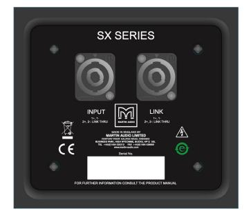
The SX112 has a pair of NL4 connectors on the rear panel. These are wired in parallel and whilst one is nominally labelled 'INPUT' and the other as 'LINK', connection in and out can be made to either connector. Connection to the drive unit(s) is made to pins 1+/-. There is no internal connection to pins 2+/- although these are linked together so can be used for example to carry a mid/top signal and connected to a full range system using a cable wired with reverse connections (pins 2 to pins 1).
