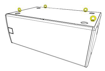
Remove the M8 counter-sunk screws and screw the eyebolts into position. We would recommend four eyebolts and an additional eyebolt as a redundant safety bond. This should be attached to a different point than the other bolts to support the cabinet in the event of the other points failing.
