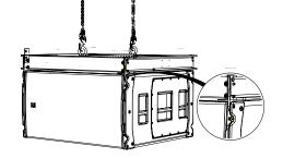
Remove the pins from the stow position, rotate the links to line up with the pin hole position on the SXHF218 above.
