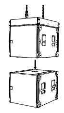
Replace the pins into the lock position on the cabinet above making sure all four links are securely attached.
