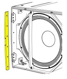
Remove the three screws from the bracket.
