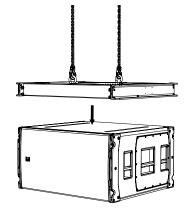
Replace the WPLGRIDt pins to link the SXHF218 securely to the WPLGRIDt. The SXHF218 pins for the first cabinet are not needed in this configuration and can be placed back in the stowed position.
