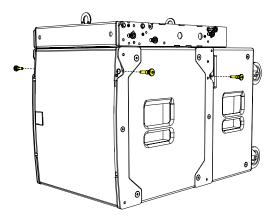
Rotate the front links and lift the rear links to align with the pin holes in the WPMSXGRIDT.
