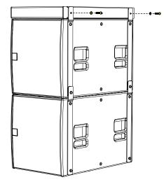
Repeat the process for the desired number of cabinets for the array.
