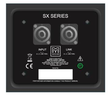
The SX118 has a pair of NL4 connectors on the rear panel. These are wired in parallel and whilst one is nominally labelled 'INPUT' and the other as 'LINK', connection in and out can be made to either connector. Connection to the drive unit(s) is made to pins 1+/-. There is no internal connection to pins 2+/- although these are linked together so can be used for example to carry a mid/top signal and connected to a full range system using a cable wired with reverse connections (pins 2 to pins 1).
