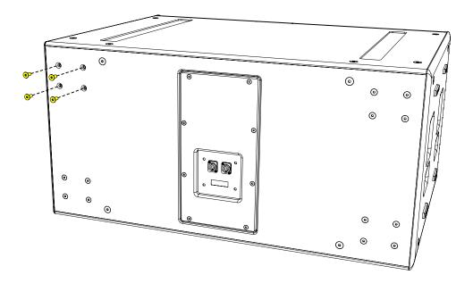
Position each castor over the insets and screw into place using the fixings supplied in the kit.
