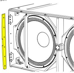
Remove the three screws from the bracket.
