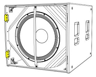
Replace the grill supports and fit the grille making sure the safety screws are replaced.
