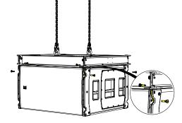
Raise the WPLGRIDt and SXHF218 to a height suitable to fit another SXHF218 below the array, lower it making sure the protective nylon skids line up and fit into the recessed channels on the SXHF218 below.
