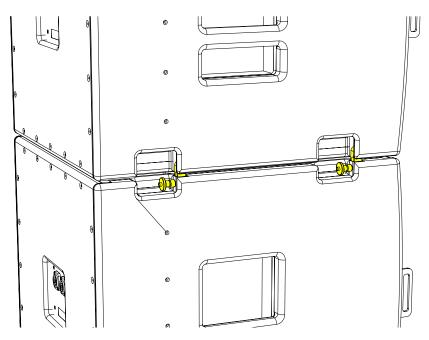
More cabinets can be added as required or transition frames connected to enable flying of either MLA Mini or WPM arrays under the SXP115. For more details see the User Guides for MLA Mini and WPM.
