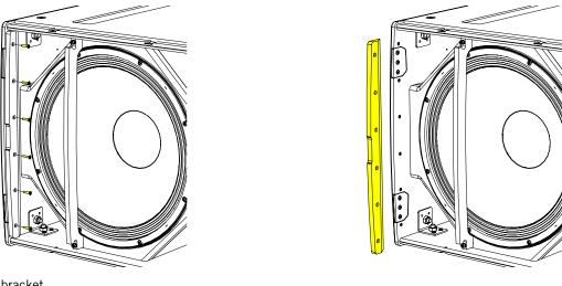
Remove the three screws from the bracket.
