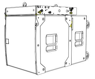
Place an SXCF115 on top and align with cabinet below. Release the pins from the cabinet below and rotate the front links. Slide the rear links up to the cabinet above.
