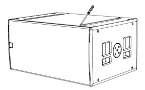
Remove the Grille and screws from the side of the cabinet and remove the grille support.
