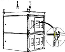
Warning: these torque settings only apply to the bolts that attach the flying brackets to the case. Don't use these settings for any other bolts, otherwise you could damage the case.
