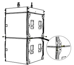
Remove the pins from the from SXCF118 to release the links. Rotate the SXCF118 links and line them up with the pin holes in the WPSGRIDt.
