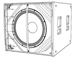
Remove the three screws from the bracket.
