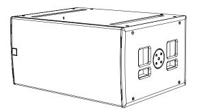
Remove the grille and screws on the side of the cabinet
