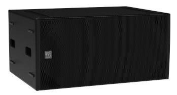
The SX215 is a powerful, compact subwoofer with an operating range of 45 - 100 Hz  $\pm$  3dB. It features two long excursion 15" (380 mm) / 4" (100 mm) voice coil drivers with water-resistant cones and triple roll surrounds, delivering exceptional low-frequency extension and impact from a compact enclosure. Eight reflex ports with a large frontal area increase LF output efficiency and reduce turbulent air noise at high levels.
