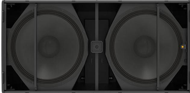
The SX218+ delivers very high output and superb transient performance with minimal distortion, so it is ideal for demanding applications. It has an operating range of 38 Hz–100 Hz  $\pm$  3 dB and houses two 18" (460 mm) long-excursion drivers with 4" (100 mm) voice coils, water-resistant cones and triple-roll surrounds. Each driver handles 1500 W AES and has a magnet structure and suspension engineered for maximum linear excursion.
