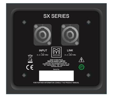
The SXF115 has a pair of NL4 connectors on the rear panel. These are wired in parallel and whilst one is nominally labelled 'INPUT' and the other as 'LINK', connection in and out can be made to either connector. Connection to the drive unit(s) is made to pins 1+/-. There is no internal connection to pins 2+/- although these are linked together so can be used for example to carry a mid/top signal and connected to a full range system using a cable wired with reverse connections (pins 2 to pins 1).
