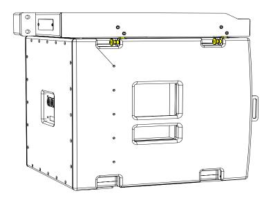
If more subs are to be linked under the first, raise the height of the first sub so you can position a second sub directly under the first. Remove the flying pins in the bottom drop-down rigging links in the first sub and lower it onto the second ensuring that the rigging links engaging all four rigging slots in the second sub exactly as you did with the frame and first cabinet.
