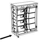
Unlatch the top from the supporting poles in four places, lift it off and set it aside.
