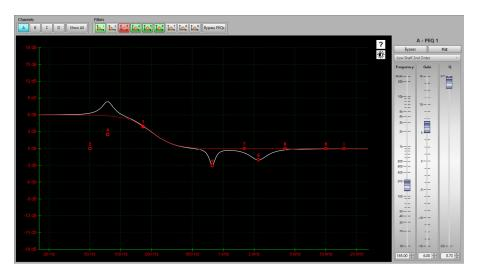
The output EQ is greyed out as it is used to apply the EQ created by your DISPLAY project, however the high-pass filter is available for adjustment so you can determine the crossover point between the WPL array and your subwoofers.
