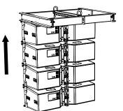
Lift the array to a height where a second cart can be placed
