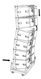
Lift the array a fraction so that there is no weight on the front rigging brackets.
