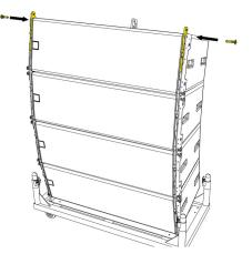
Insert a rigging pin at the front rigging position on each side.
