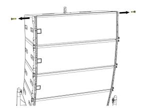
Raise the front rigging brackets on the fifth cabinet and insert a rigging pin on both sides in the fourth cabinet.
