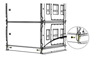
Replace stow pins to link position on the bottom of the SXHF218, making sure all four corners are secure.
