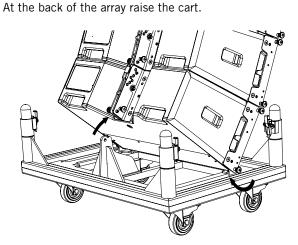
Remove the LOCK pins from the rear rigging bracket on the bottom four cabinets.  $% \left( {{{\rm{DCK}}}} \right) = {{\rm{COCK}}} \right)$
