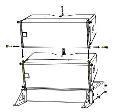
Insert the link pin in the lowest hole to secure the rear of the WPS.
