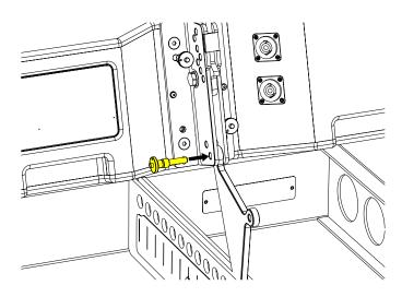
Secure the front of the second cabinet with link pins on both sides.
