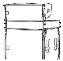
Fit the ground-stack bar into the appropriate hole in the central spine of the flying frame. Note that the orientation of the bar and the correct hole to use in the frame will be determined by the angle of the first WPS cabinet in the stack and will be calculated by the DISPLAY project.
