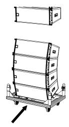
Lower the array and align the front rigging assemblies of the fourth cabinet with the front rigging points of the fifth cabinet.
