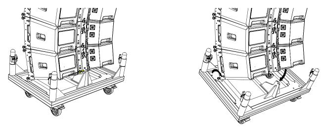
Repeat at the front of the array supporting the cart and removing the pins holding the cart to the array.
