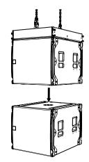
Replace the pins into the lock position on the cabinet above making sure all four links are securely attached.
