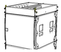
Remove the link pins and lower the WPS cabinet onto the frame until the two up-right bars on the frame locate in the front rigging assembly of the WPS. Insert the link pins in the WPS rigging assembly to secure the front rigging system.
