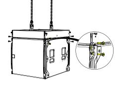
Replace the pins to link and lock the SXCF118 securely to the WPSGRIDt.
