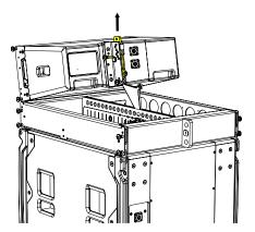
Repeat the process for the second cabinet, removing the link pins and lower it onto the first cabinet.
