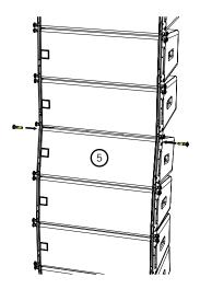
The cabinet angles will open as far as the pins will allow to the angle that has been pre-selected. Insert rigging pins at the LOCK position on the remaining cabinets.
