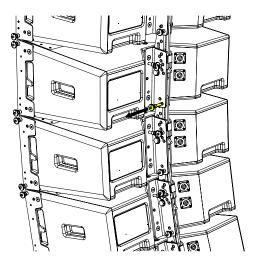
Remove the front locking pins from the fifth cabinet at each side. Ensure the cart is fully grounded when removing pins.
