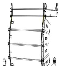
Insert the pin into the LINK hole on the flying frame.
