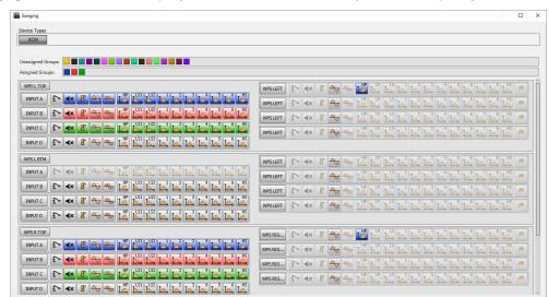
Comprehensive ganging is available so for example you can ensure that stereo arrays remain completely identical.
