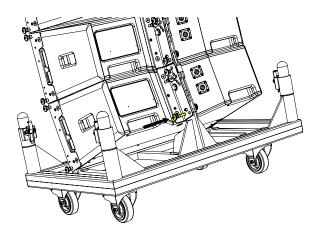
Lower the array until the cart is on the ground taking the weight of the array allowing the cabinets to collapse down until the trapezoidal sides are touching.
