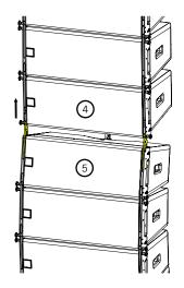
Remove the link pins from the fourth cabinet (the front links return to the transport position). Stow the pins and replace the poles and lid ready for transportation.
