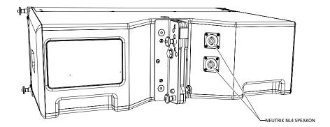
The two NL4s are wired in parallel so either can be used as a nominal 'input' or 'link' output. WPS is a passive system and all speaker cables and link cables must utilise 2-core cable.
