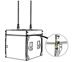
Remove the pins from the stow position, rotate the links to line up with the pin hole position on the SXCF118 above.
