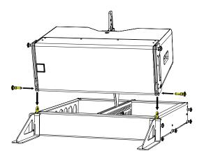
Remove the lock pins from the rigging assembly and raise the link bar. Replace the lock pins to hold the bars in the up position.
