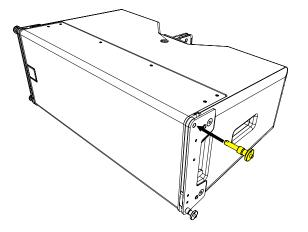
It is important to check that the central button does not remain depressed once you have put it in place as this would indicate that the pin has not been pushed all the way into position and the ball bearings at the end of the pin have not been able to pop out and rigging the pin in place. If the pin is not locked the array is unsafe. The pin MUST be repositioned until it is securely locked in place.
