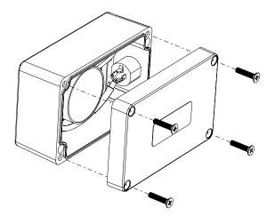
Using the PZ2 Pozidrive screwdriver, unscrew all four lid screws until the lid can be removed from the base of the box. Note that the screws do not have to be completely removed from the lid, they can remain captive in the lid to prevent them getting lost.
