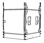
Lift the front links on the left and right of the WPS and pin in position.
