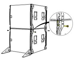
Remove the pins, rotate the links to line up and align with the pin hole position on the WPSGRIDt.
