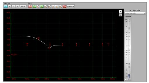
The output EQ is greyed out as it is used to apply the EQ created by your DISPLAY project, however the high-pass filter is available for adjustment so you can determine the crossover point between the WPS array and your subwoofers.
