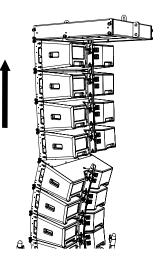
Swing the bottom four cabinets (which will now be a rigid array due to the rigging pins) backwards until butted against the upper half of the array.
