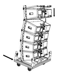
Lift the array so that the front links are floating. This makes it easier to remove the linking pins from the fourth cabinet.
