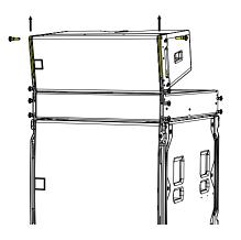
Raise the rear link into place and pin it at the desired angle.
