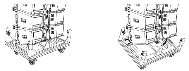
Repeat at the front of the array supporting the cart and removing the pins holding the cart to the array.
