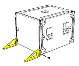
Replace the pins into the lock position on the cabinet above making sure all four links are securely attached.
