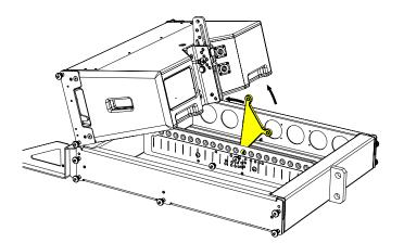
Repeat the process for the second cabinet, removing the link pins and lower it onto cabinet 1.
