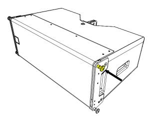
Pull the pin clear using the wide flange whilst your thumb depresses the central button.
