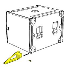
If needed place a second SXCF118 on top and remove the pins from the stow position, rotate the links and align them with pin holes on the top cabinet.
