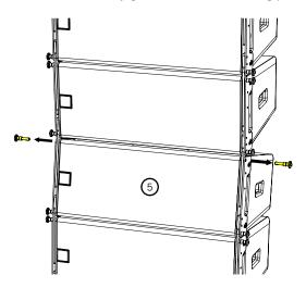
Lift the array and allow it to swing on the front link. The lower the array down so that the cart meets the floor.
