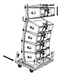
Insert a pin in the rear rigging bracket at the correct angle. Allow the bottom four cabinets to swing back down and insert rigging pins into the LINK and LOCK positions on the fourth cabinet. Connect the cable loom and any link cables as required to the lower four cabinets.
