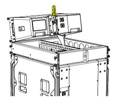
Secure the front of the second cabinet with link pins on both sides.
