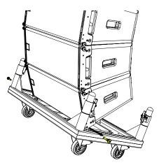
Once the cart is removed the four supporting poles can be placed in the base and the top fitted directly to the base and the two clipped together. The assembly can now be moved to a suitable location for storage.
