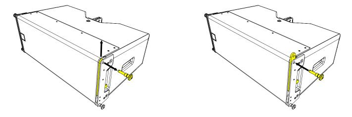
Inter-cabinet angles are set using the rear rigging assembly. This consists of a link bar with indexed holes which can be moved upwards and secured with a link pin in one of eight available positions: 0.5°, 1°, 2°, 4°, 6.5° and 10°.
