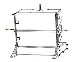
Lift the rear link of the first cabinet and insert a link pin in the hole for the angle required as indicated in the DISPLAY prediction. Lift the back of the second cabinet until the angle is reached and insert a lock pin in the LOCK position to hold the cabinet at the required angle .
