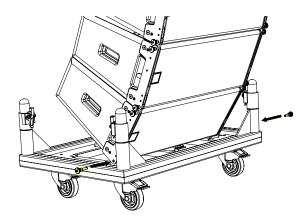
Pin the cart to the rear rigging bracket of the array.
