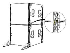
Replace the pins locking the link into the WPSGRIDt.
