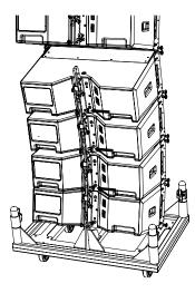
Raise the array clear of the transport cart, allowing access to the rear of the array.
