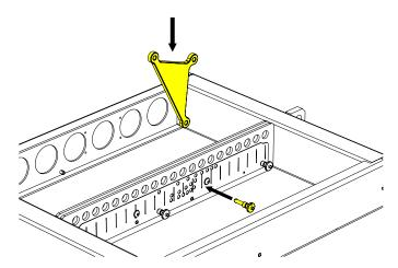
Remove the link pins and lower the WPS cabinet onto the frame until the two up-right bars on the frame locate in the front rigging assembly of the WPS. Insert the link pins in the WPS rigging assembly to secure the front rigging system.
