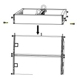
Insert the link pin at the front rigging position on each side.
