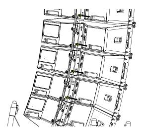
Raise the front of the cart and pin it in position to the front of the array.
