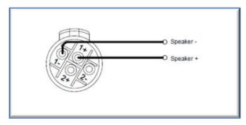
Additionally, the channel 2 output is duplicated on the speakON connector for amplifier channel 1 for bi-amp wiring. Similarly, the channel 4 output is duplicated on the speakON connector for amplifier channel 3. This can be useful for making a connection to two loudspeakers with one 4-core cable (i.e. bi-amp).
