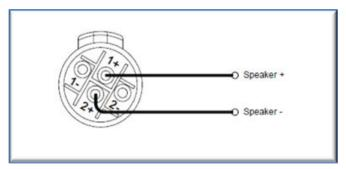
More than one speaker can be connected to each channel provided the total impedance per channel is 2 ohms or more. In bridged mode (page 24) the minimum total impedance is 4 ohms.
